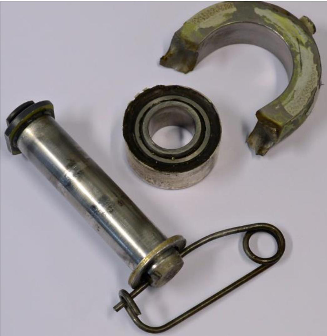
Figure 4: Upper forward suspension bar fitting. Photo: AIBN
