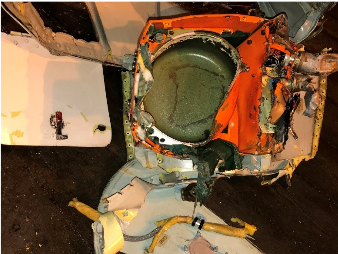
Figure 5: The destroyed Flight data recorder. Photo: AIBN
