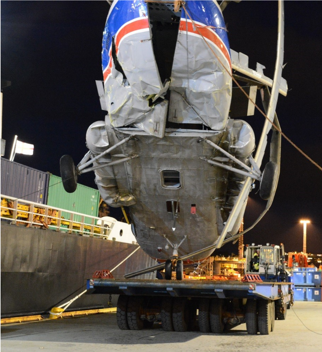
Figure 6: Damage to the underside of the helicopter. Photo: AIBN
