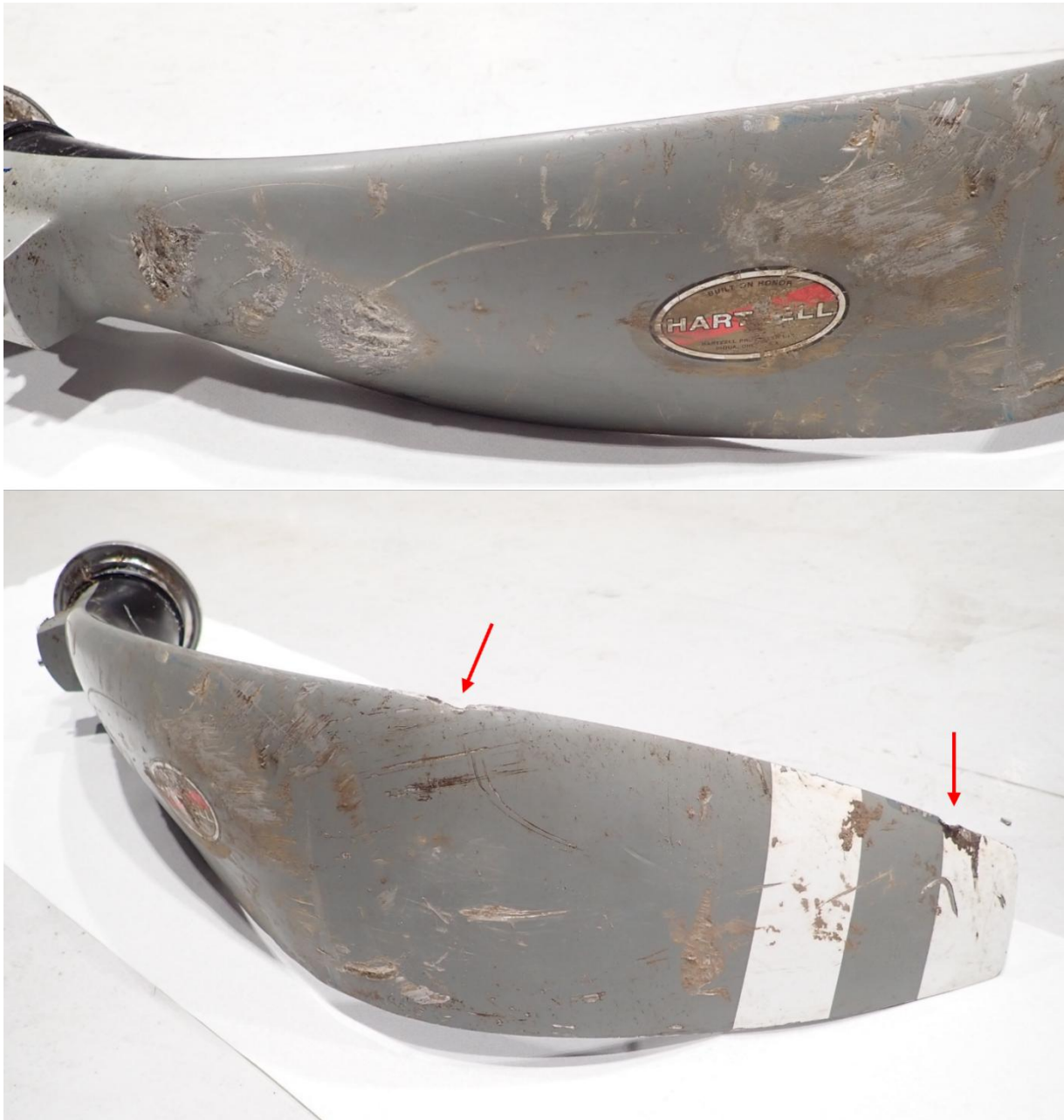
Figure 16: Propeller blade no. 2 from LN-TBN. Red arrows indicate two significant cuts in the leading edge of the blade. Photo: NSIA
