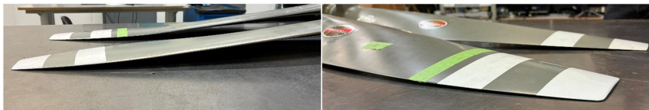
Figure 15: Propeller blade no. 1 from LN-TBN (marked with green tape) placed next to a propeller blade of the same type shows that the outermost part of the blade is bent forwards. Photo: NSIA
