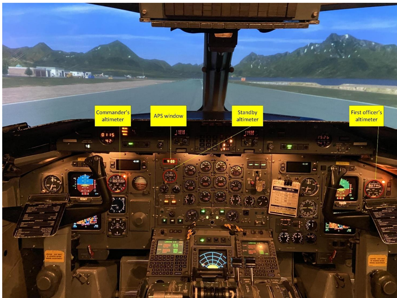
Figure 2: Location of the barometric altimeters in a DHC-8-100. Photo and labelling: NSIA
