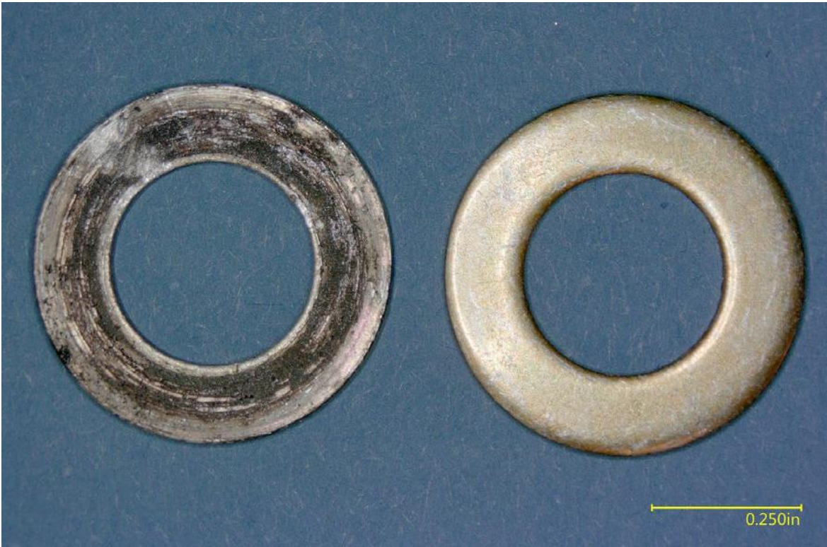
Figure 14: The washer found in the main gearbox on the left, and the reference washer on the right. Photo: NTSB/NSIA
