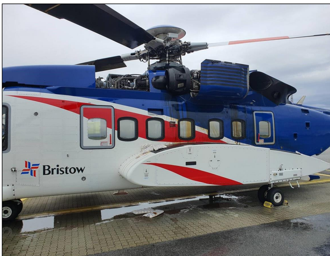
Figure 3: LN-ONQ shortly after landing. Visible oil spill on the left side of the fuselage and open cover plates around the left engine and main gearbox. Photo: Bristow Norway / NSIA
