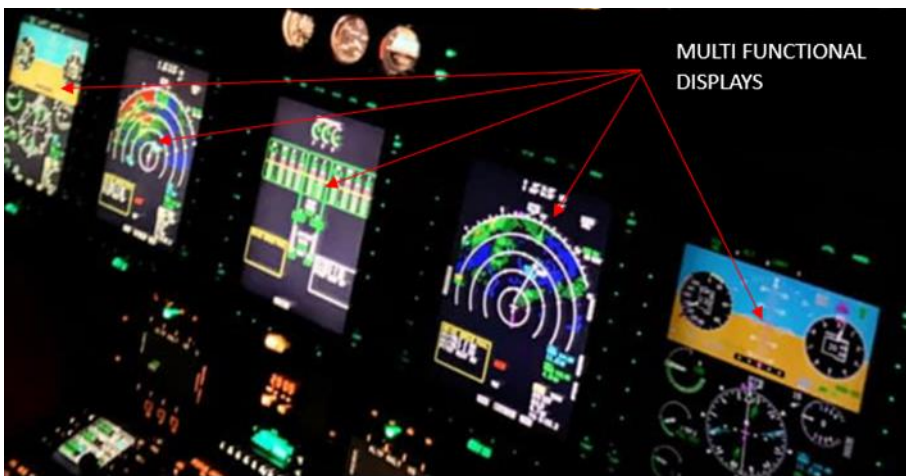
Figure 8: Five multi functional displays in the cockpit of the S-92. The information to the crew regarding the main gearbox oil pressure and temperature is displayed on the MFD in the middle. Image: Brita Sandveen. Illustration: NSIA
