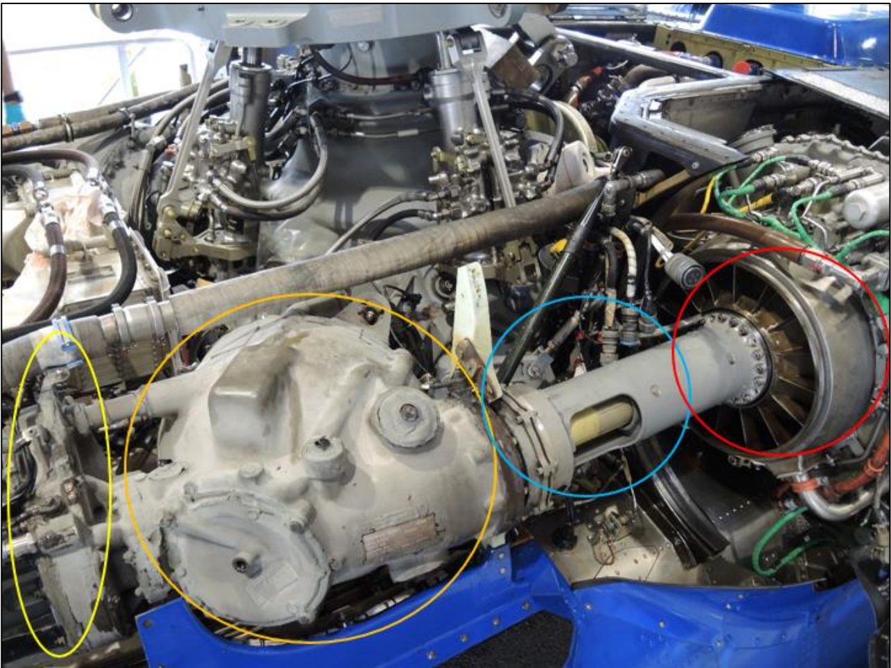
Figure 6: LN-ONQ photographed the day after the incident. Left accessory module (on the far left, yellow circle) and the left input module (in the centre, orange circle). The drive shaft (blue circle) and the front of the left engine (red circle) can be seen on the right. Photo: NSIA
