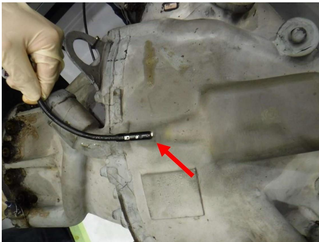
Figure 12: Left input module seen from below. The connection for the main gearbox module can be seen on the left side of the photo. The end of the borescope (the flexible inspection equipment) is laid over the passageway that was followed into the washer. The red arrow indicates where the washer was found. Photo: NTSB/NSIA
