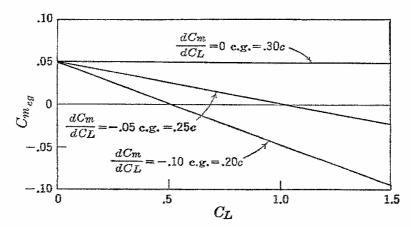
FIGURE 5-18. Typical effect of e.g. shift on pitching moments.
