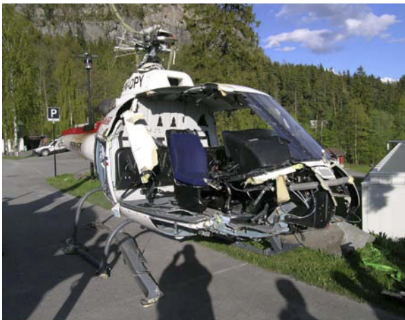
Figure 7: The damaged right side of the cabin.
