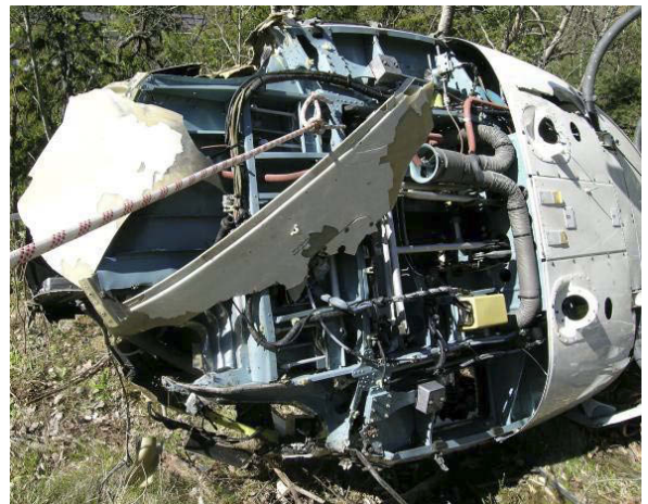
Figure 8: Damage forward and under the helicopter.
