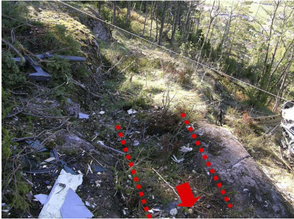
Figure 5: The ledge where LN-OPY made an emergency landing. The dotted lines show the position of the helicopter's landing gear. The arrow shows the direction of the helicopter before it tipped over.
