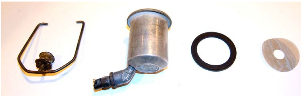
Figure 4: Parts of the gascolator assembly: Fastening clamp, bowl with drain nipple, gasket, filter
