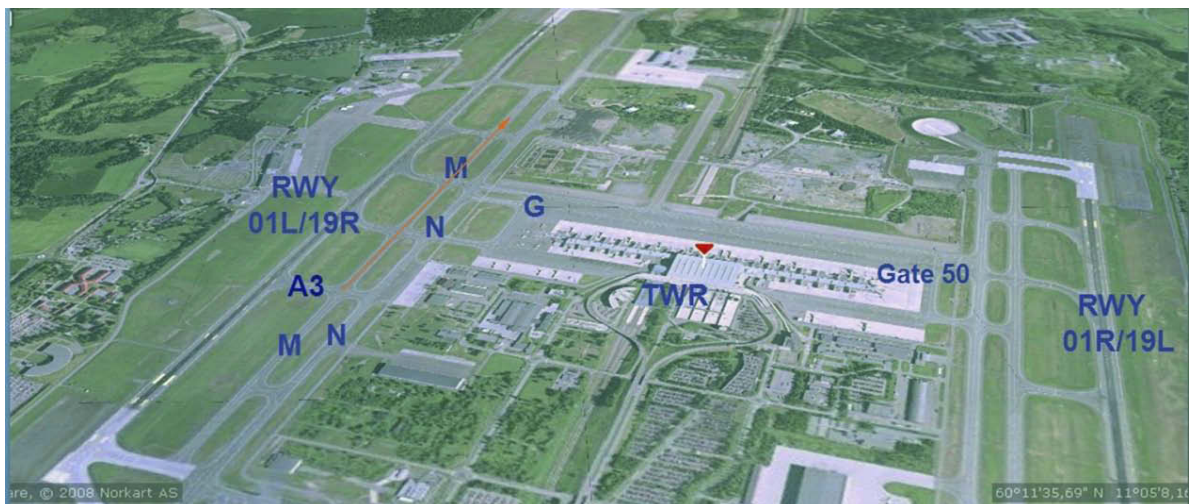
Figure 1: Oslo Airport Gardermoen, (ENGM). The orange line indicates where the aircraft took off northbound on taxiway M, instead of on runway 01L, west of taxiway M. See also the copy of Jeppesen's airport map in Appendix B.
