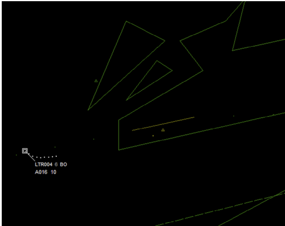
Radar print-out at 14:41:45Z. Position approx. 4 nm NM west of runway 07 threshold, altitude 1 600 ft, ground speed 100 KGS in approx. 30 kt of tailwind, course north-west through Localizer.
