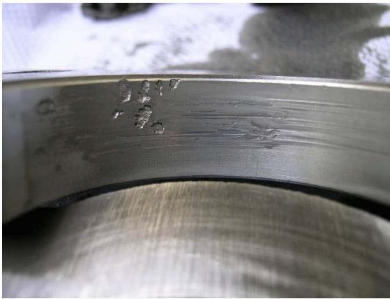
Figure 10: Damage to the crankshaft's journal bearing no. 1.
