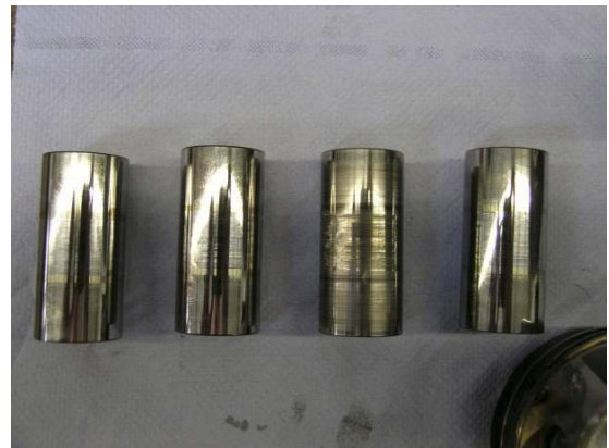
Figure 15: The colors on the gudgeon pins indicate overheating.
