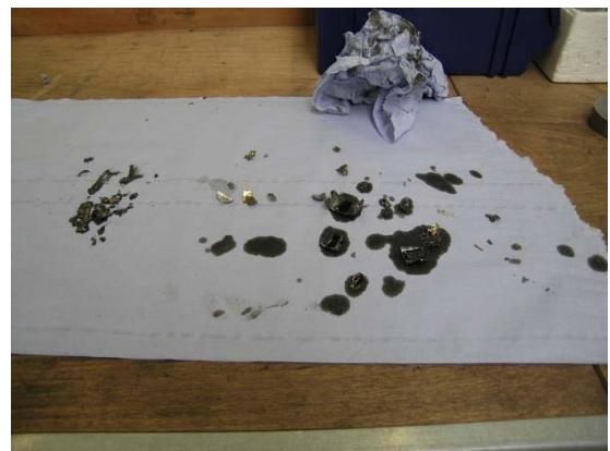
Figure 13: Small and large metal debris were discovered in the oil pan and oil filter unit.
