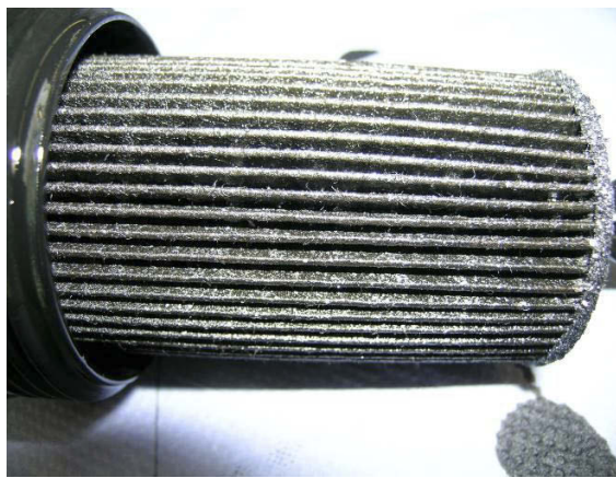
Figure 7: The engine oil filter contaminated by metal particles.
