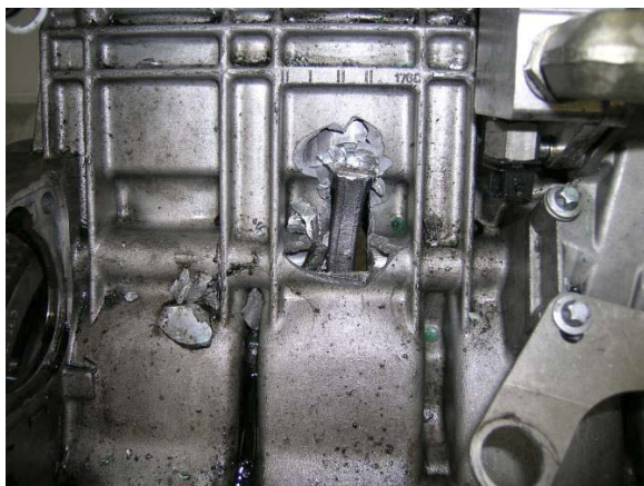
Figure 6: The left-hand side of the engine with the connecting rod sticking out.
