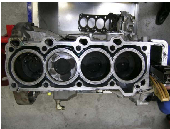
Figure 8: Picture viewing down into the cylinders. The piston in cylinder no. 3 (no. 2 from the left) was slightly damaged as a result of the impact with the cylinder head.
