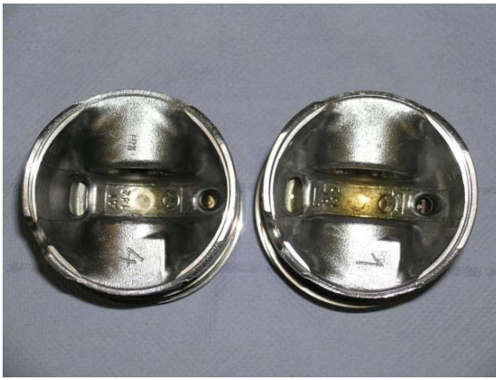
Figure 16: Color difference. Piston which has run for 1000 hours (reference piston) to the left and piston no. 1 from LN-NEX to the right.
