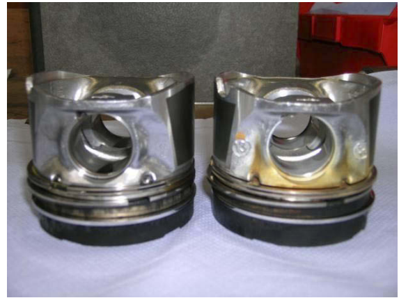
Figure 17: Color difference. Piston which has run for 1000 hours (reference piston) to the left and piston no. 1 from LN-NEX to the right.
