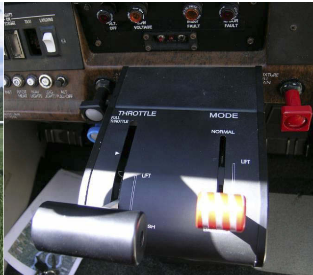
Figure 2: Throttle, mode handle and warning lights.
