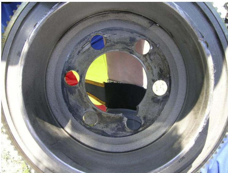
Figure 6: Starting gear ring with fretting and imprint from tilting.
