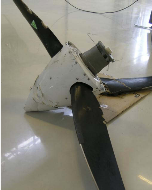
Figure 3: The propeller in the state it was found.
