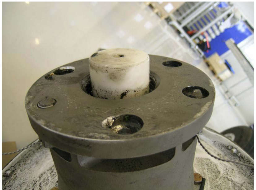
Figure 4: The propeller's mounting flange on which two of the Three remaining bolts can be seen. The locking wires are still attached to the bolt heads. Minor fretting marks can be seen on the outer diameter.
