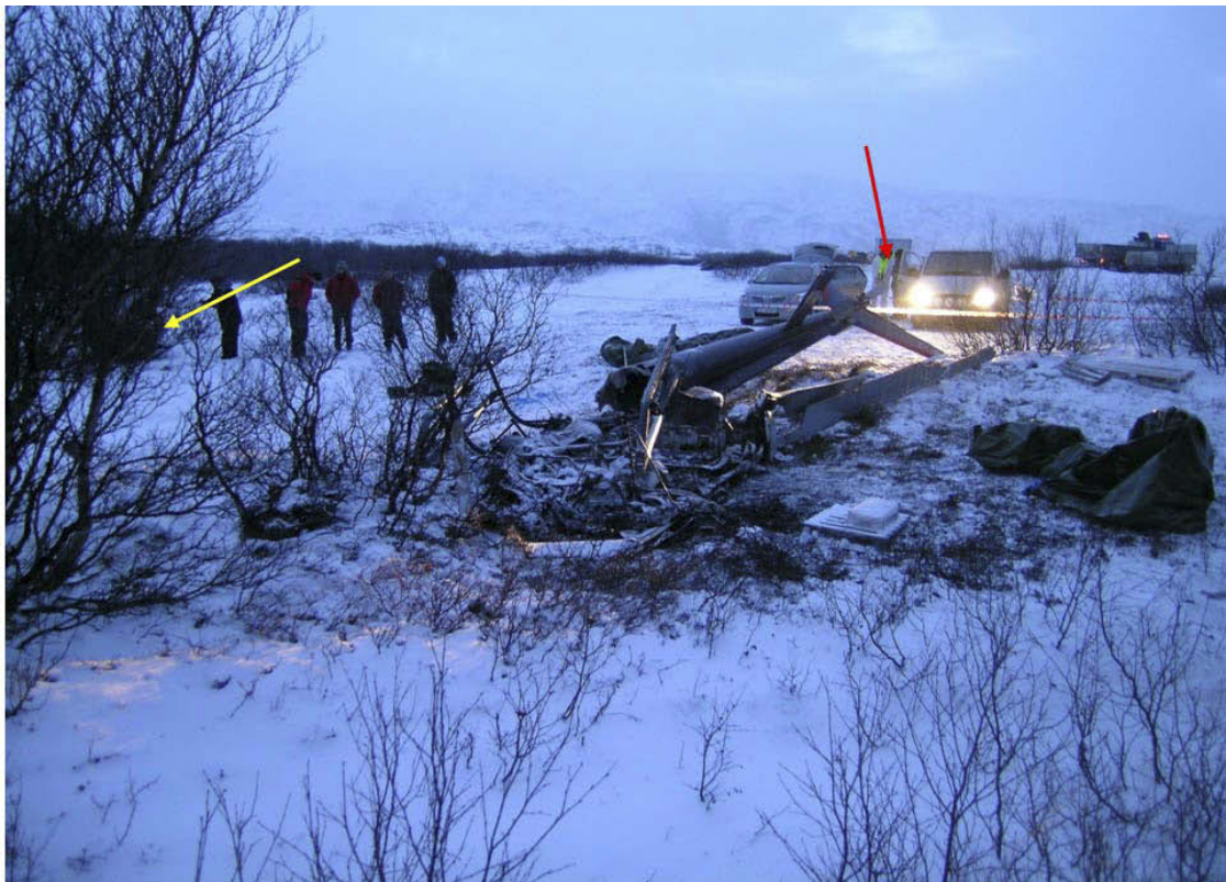
Figure 4: The helicopter wreckage seen towards the southwest. The plan was to put the excavator part down in front of the container (red arrow). The excavator ended up next to some trees by the persons in the picture (yellow arrow). Photo: AIBN
