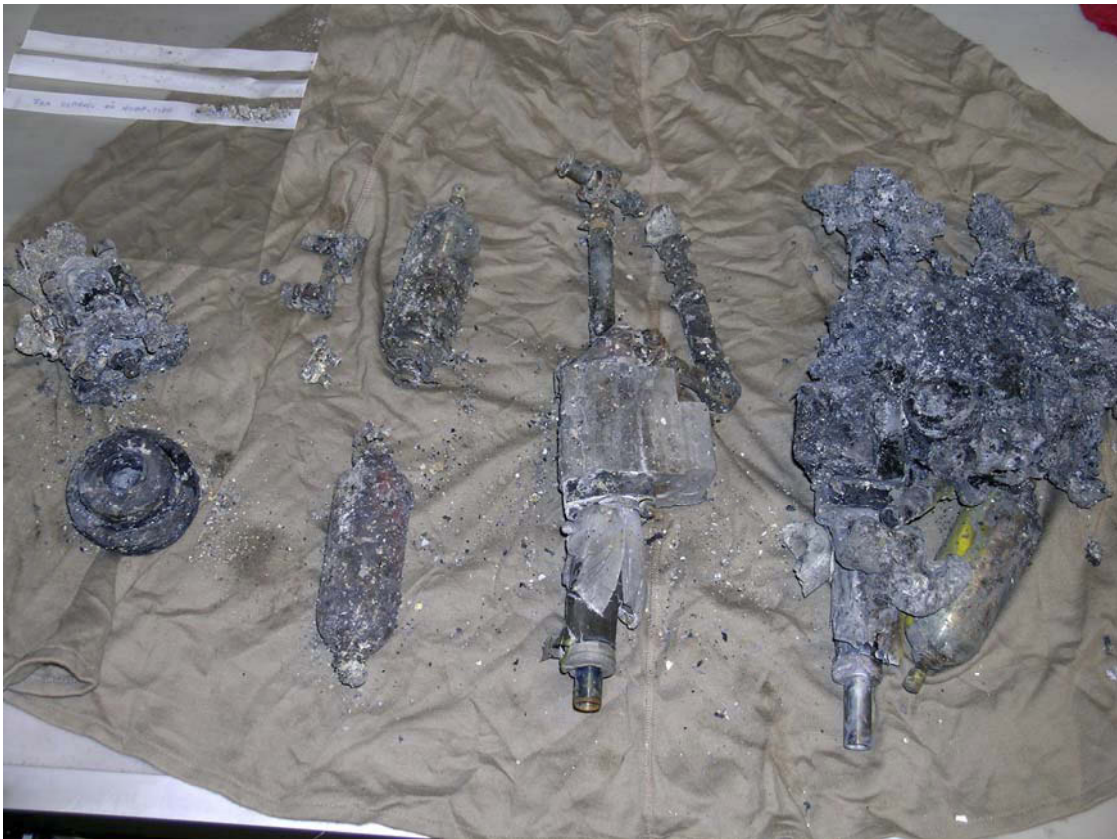
Figure 5: From left to right: hydraulic pump with driving wheel, two accumulators, servo without accumulator and complete servo with accumulator. Photo: AIBN
