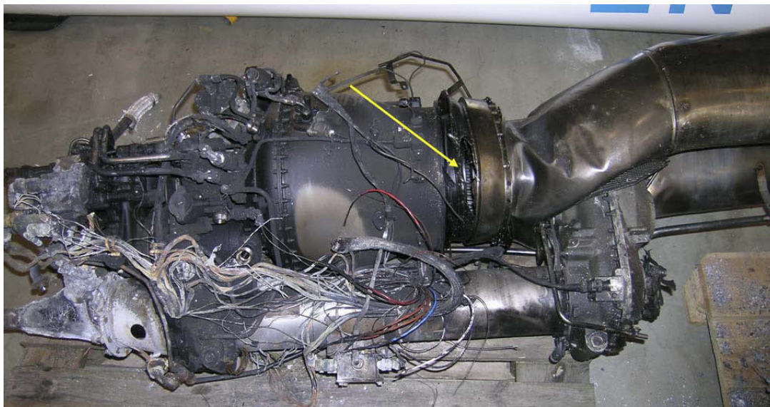
Figure 6: Engine with soot marks. Yellow arrow pointing to the tear where the turbine blades exited. The protection ring is directly to the right of the tear. Photo: AIBN
