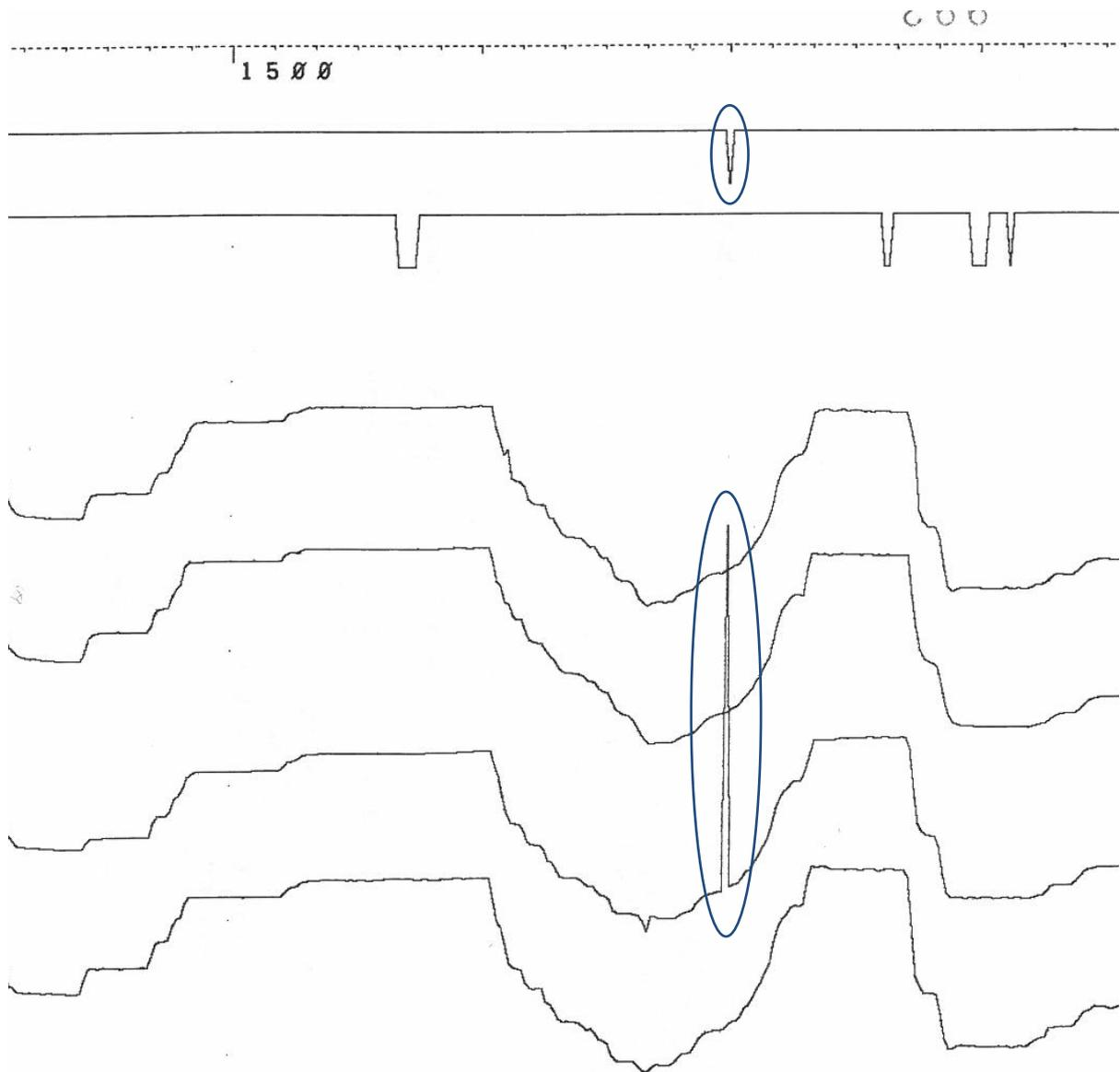
Flight Data Recorder graphs from the previous flight (Trondheim to Namsos). The sudden peak on the performance graph for engine number two (E2TORQ) and the coincident peak on the radio no. 2 (VHF2) are circled in.
