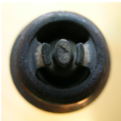
Figure 7: Examples of worn spark plugs. Photo AIBN
