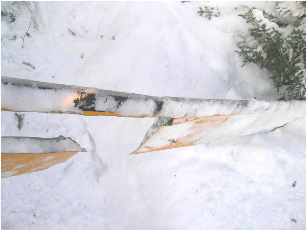
Figure 6: The upper side and leading edge of main rotor blade A with frozen snow/ice. The spar has partially separated from the rest of the blade. Photo: AIBN
