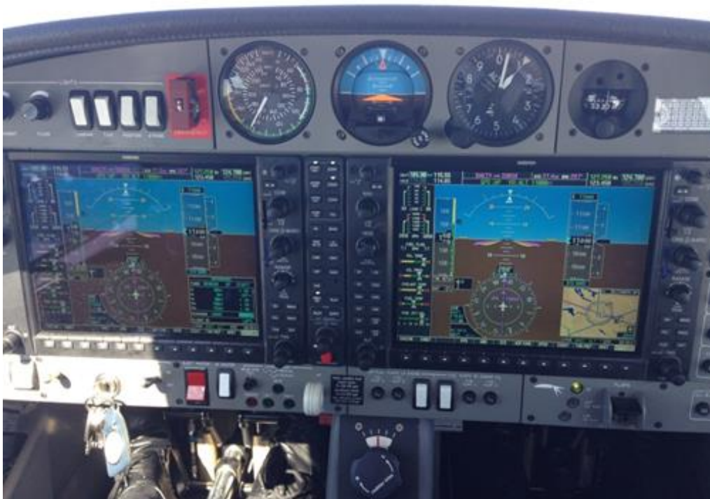
Figure 4: LN-FTL cockpit with Garmin G1000 Integrated Flight Deck System. The image related to the Traffic Advisory System (TAS) is in the lower right hand corner of the right hand screen (MFD). See close-up image in figure 5. Photo: LN-FTL Commander
