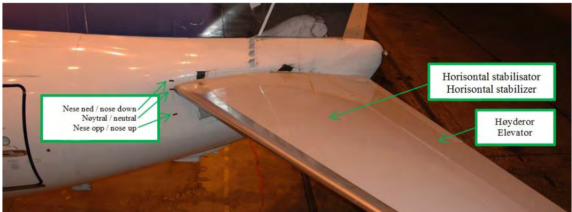
Figure 3: Shows the size ratio between the horizontal stabiliser and the elevator, as well as the range of motion for the horizontal stabiliser. Photo: AIBN
