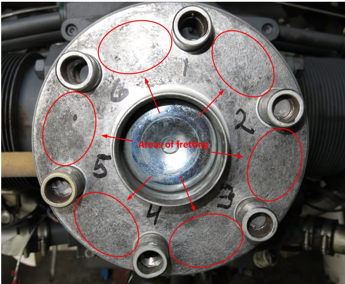
Figure 4: Areas with fretting on the crankshaft flange. Photo: AIBN
