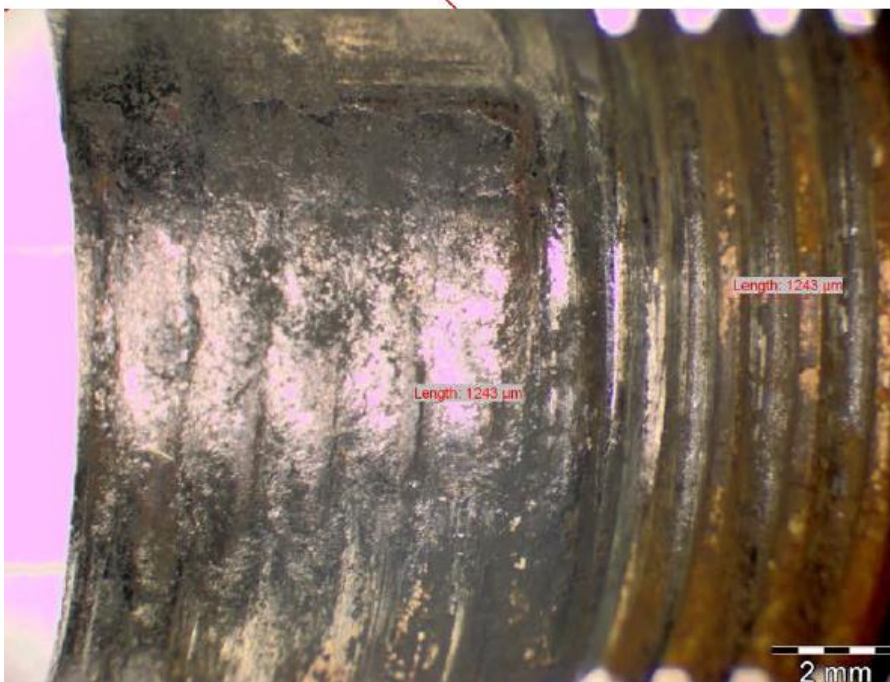
Figure 6: Traces of bolt threads in bushing. Photo: FLO materials lab
