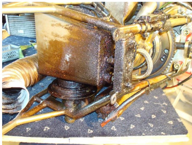
Figure 6: Fire/heat damage to the oil tank and the area near the rear engine mount. Photo: S/NLF
