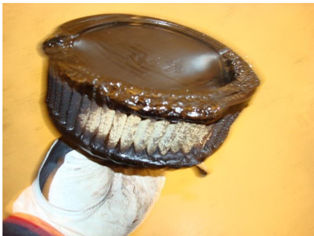
Figure 5: Fire/heat damage on the air filter. The end wall of the filter has a concave deformation. Photo: S/NLF
