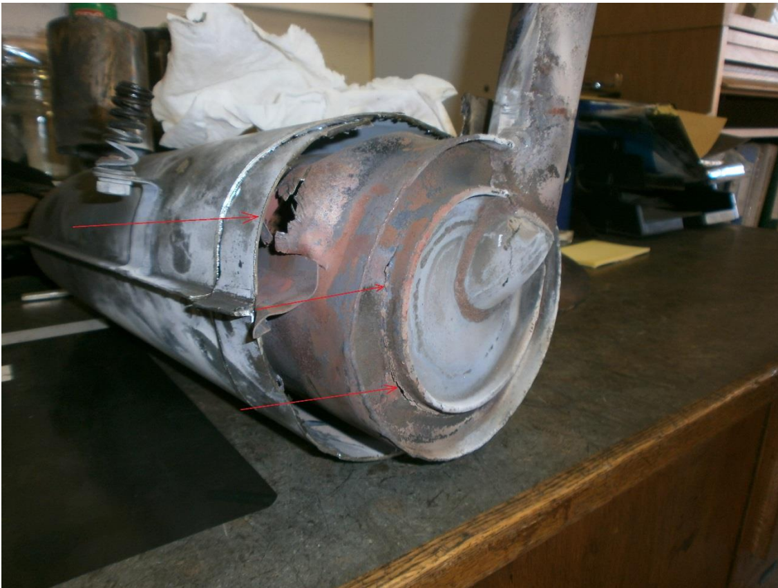
Figure 4: The exhaust silencer partially cut open. The external heat shield was first dismantled. The picture clearly shows the surrounding space where the cooling air passes through. The arrows indicate the cracks in the innermost element. Photo: S/NLF
