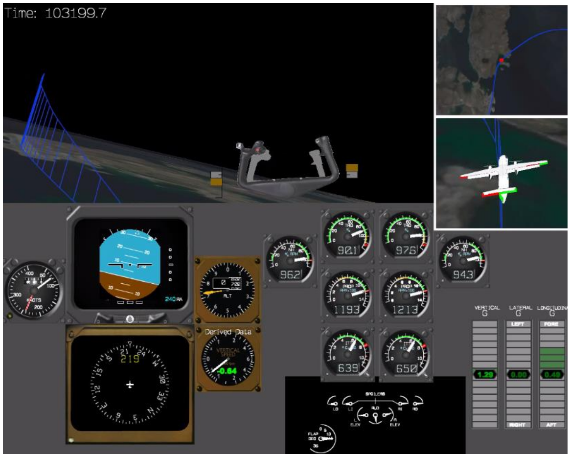
Figure 10: Freeze-frame from the animation of the incident involving LN-WIU which shows the situation as engine output nears "Full power" just before the control column is pushed resolutely forward. Note: The animation is based on data from FDR. Surroundings, visibility and wind conditions are not representative for the incident in question, and the indications from the altimeter and vertical speed indicator do not correspond with what was shown in the cockpit. Screenshot: AIBN
