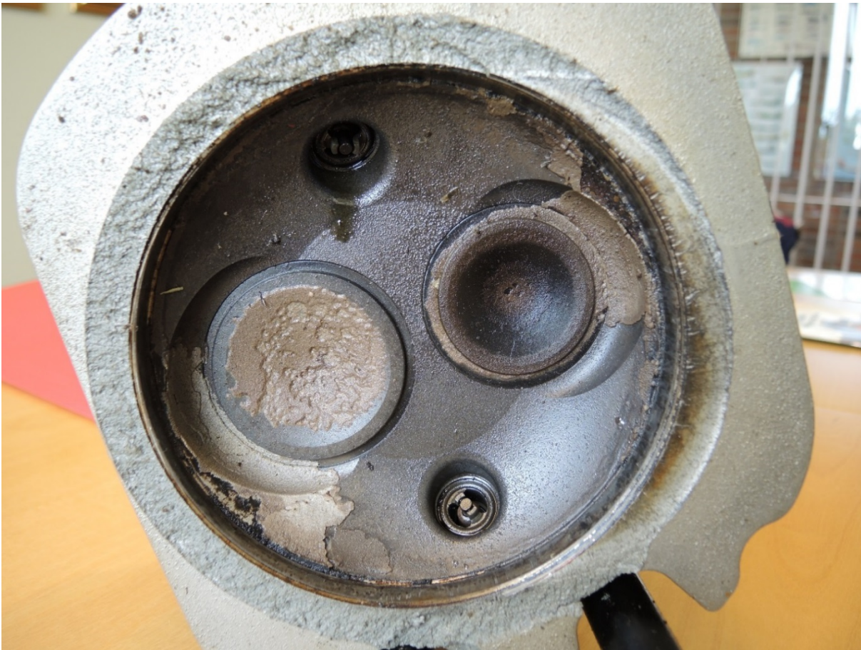
Figure 2: Fracture after the cylinder head was removed. The fracture started on the right side of the photo. Soot colour in the right side of the fracture surface shows that the fracture has been open in this area for a while. Photo: AIBN
