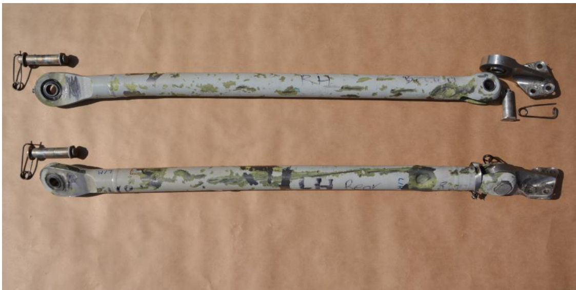
Figure 3: MGB Right and left hand aft suspension bars with attachment fittings. Photo: AIBN
