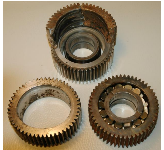
Figure 6: Parts from second stage planet gear. (The fractured gear is placed on top of a sample gear that was not involved in the accident.) Photo: AIBN
