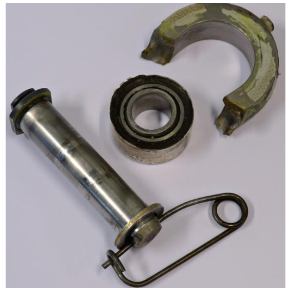
Figure 4: Upper forward suspension bar fitting. Photo: AIBN
