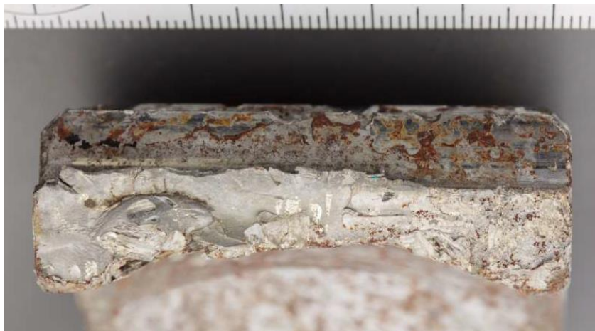
Figure 31: The cleaned through-thickness fracture surface. The cleaning was performed using a combination of acetate replica stripping and inhibited HCl solution with ultrasonic agitation. Macro marks (beach marks) are visible towards the upper edge of the gear (left hand side in photograph). Photo: AIBN/QinetiQ
