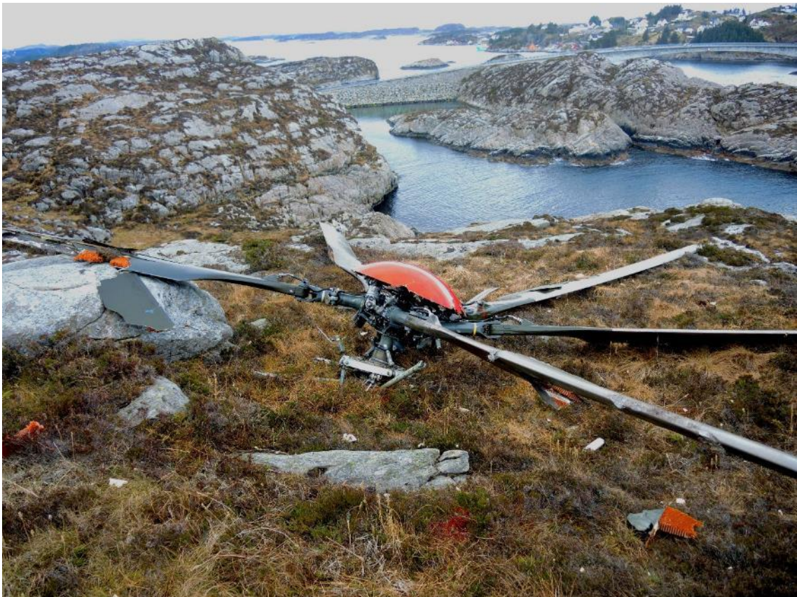
Figure 24: The main rotor and rear suspension bars as found at the island Storskora. Photo: AIBN
