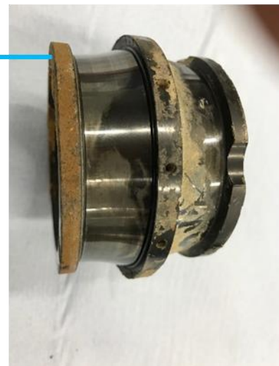
Figure 50: The inner race of the fractured planet gear after cleaning of the upper race (left in photo). Position on the carrier is given by the arrow. Photo: AIBN/QinetiQ
