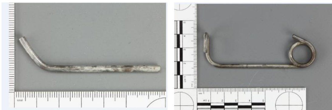
Figure 55: Two segments of safety pins found near the rotor mast. Metallurgical examination proved these to be from two different pins. Photo: AIBN/QinetiQ
