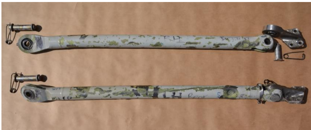
Figure 54: Left and right aft suspension bars with clevis pins, safety pins (only one shown in each position) and fuselage fittings. Both suspension bars have indentations from gear teeth. Photo: AIBN
