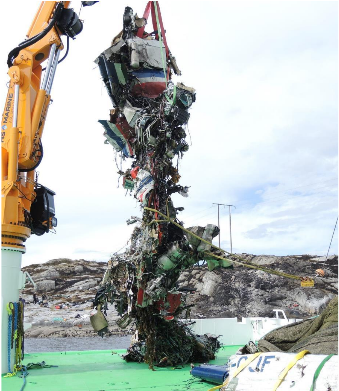
Figure 22: The main wreckage during recovery. The tail boom seen at the lower right had already been recovered. Photo: AIBN
