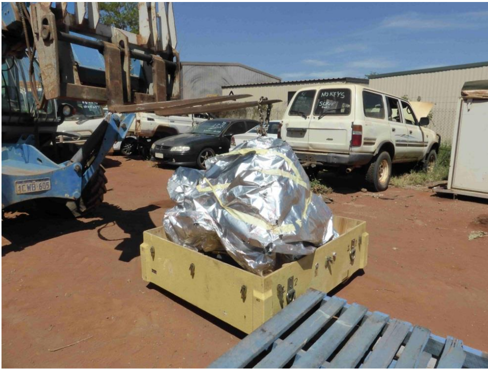
Figure 13: MGB in transport container after the transport accident. Photo: Airbus Helicopters
