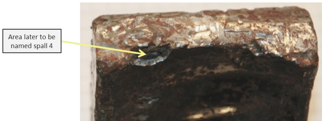
Figure 28: The fracture surface to the left in Figure 27, in general other surfaces appeared to be ductile overload, however, this surface indicated by the yellow arrow was of particular interest. Photo: AIBN/NDL
