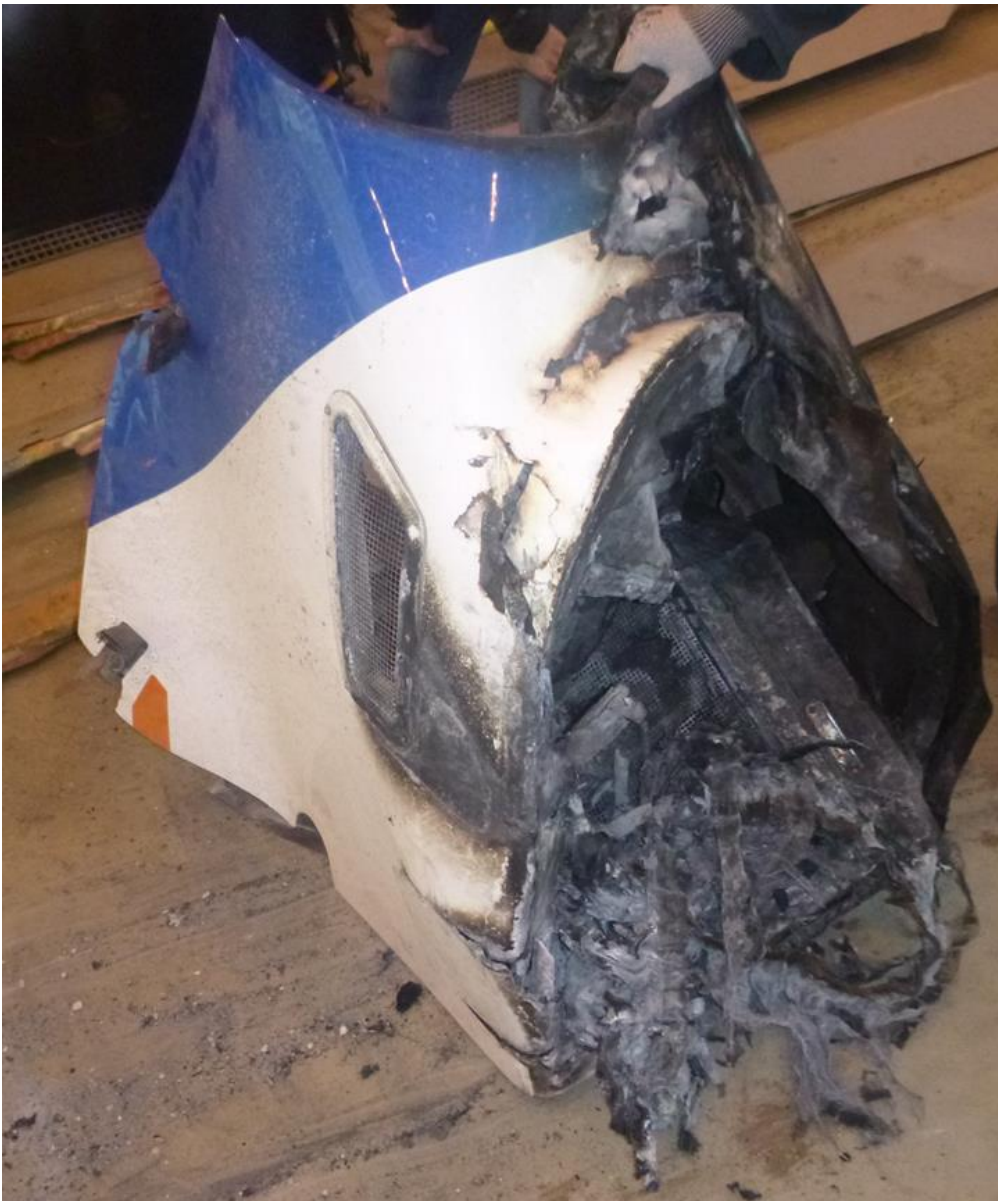
Figure 7: Engine cowling with incinerated air intake filter. Photo: AIBN
