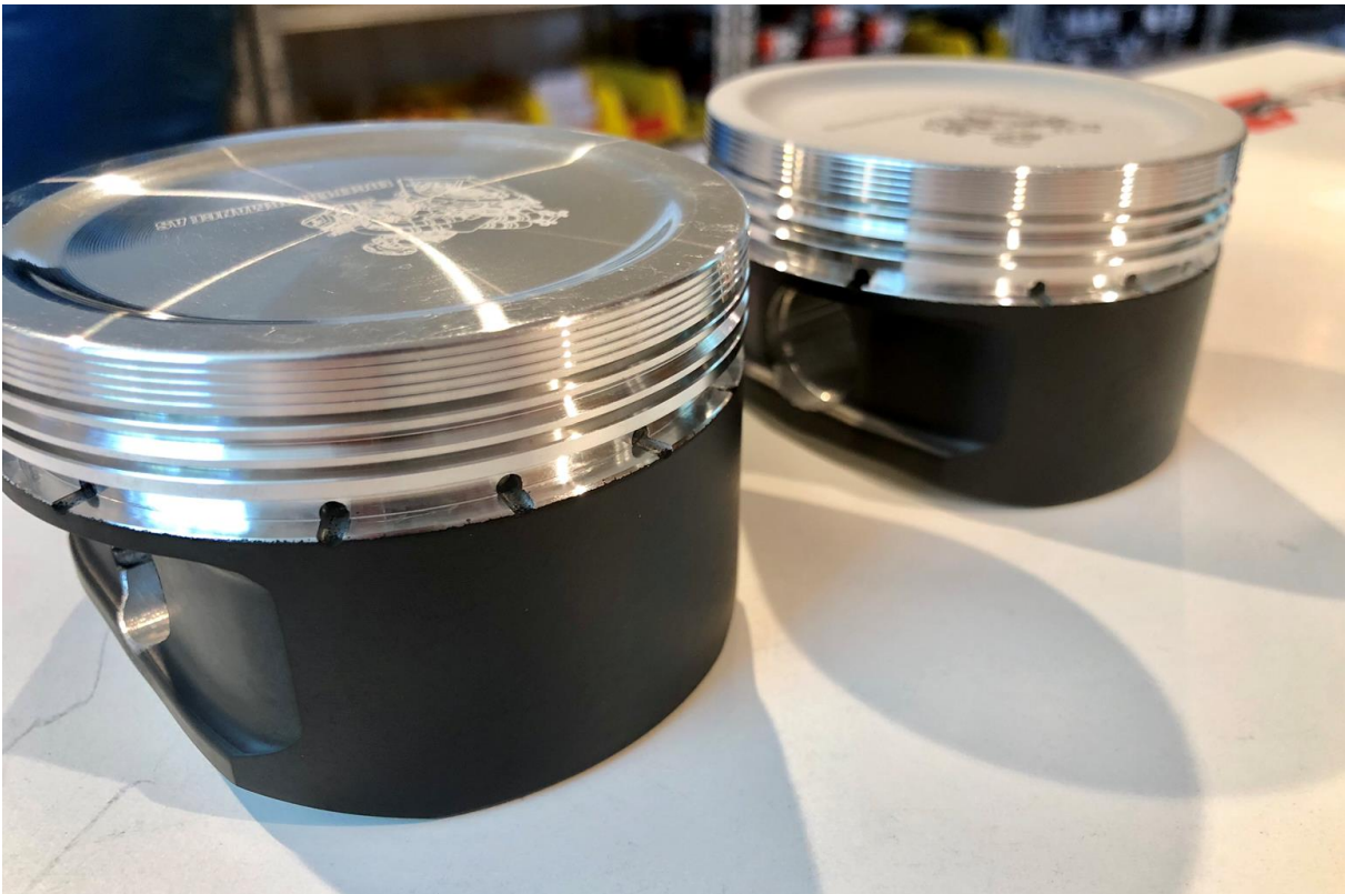
Figure 19: New design of «Big Bore» pistons. Photo: EdgePerformance
