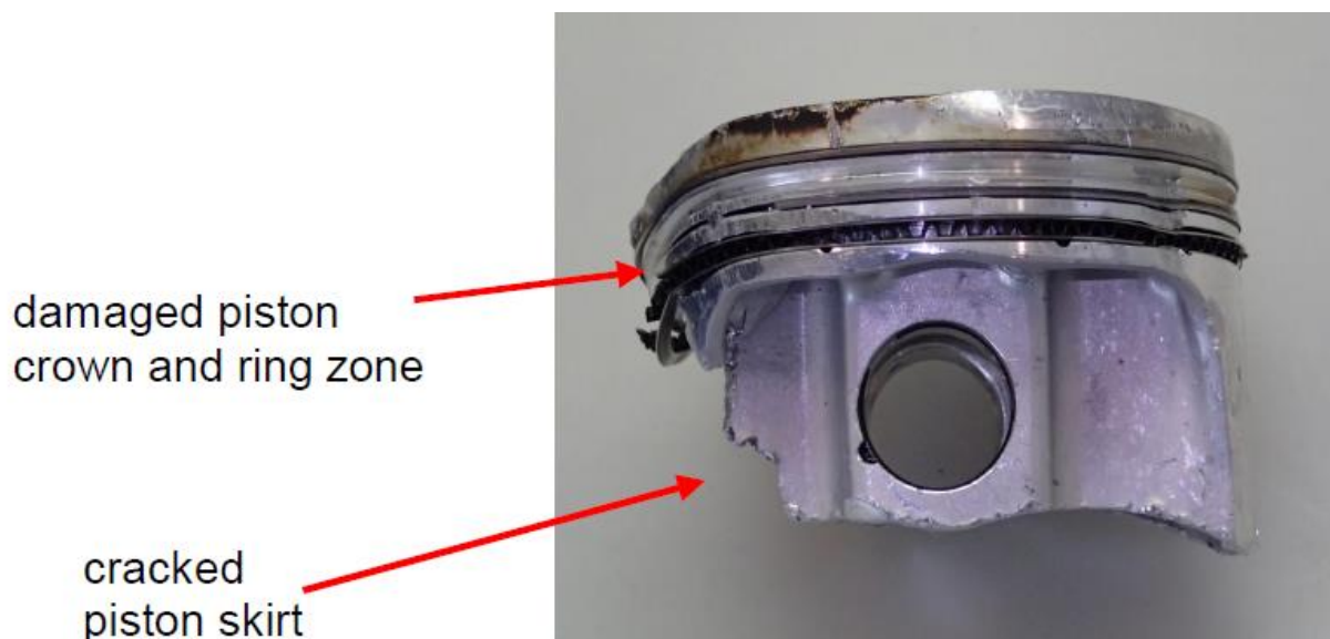
Figure 6: Damages on piston no. 2. Source: Rotax
