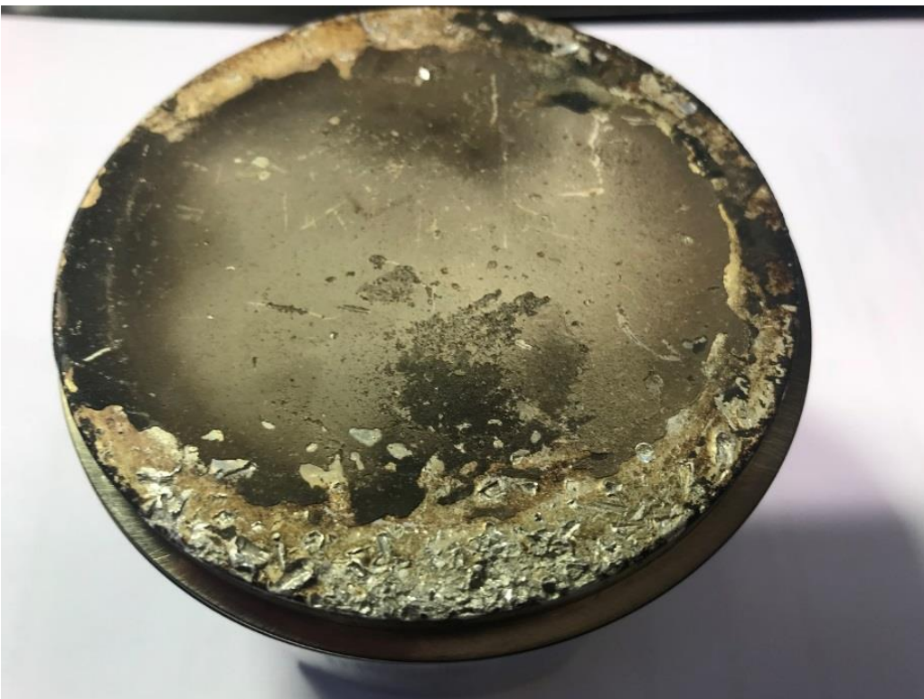
Figure 9: Damages to the piston crown of piston no. 4. Photo: AIBN
