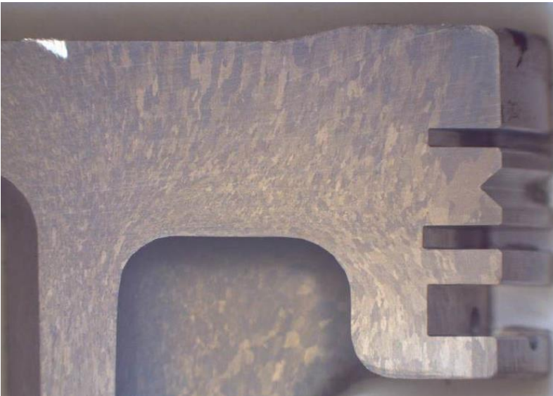
Figure 17: Coarse granular structure in pistons. Photo: Rotax
