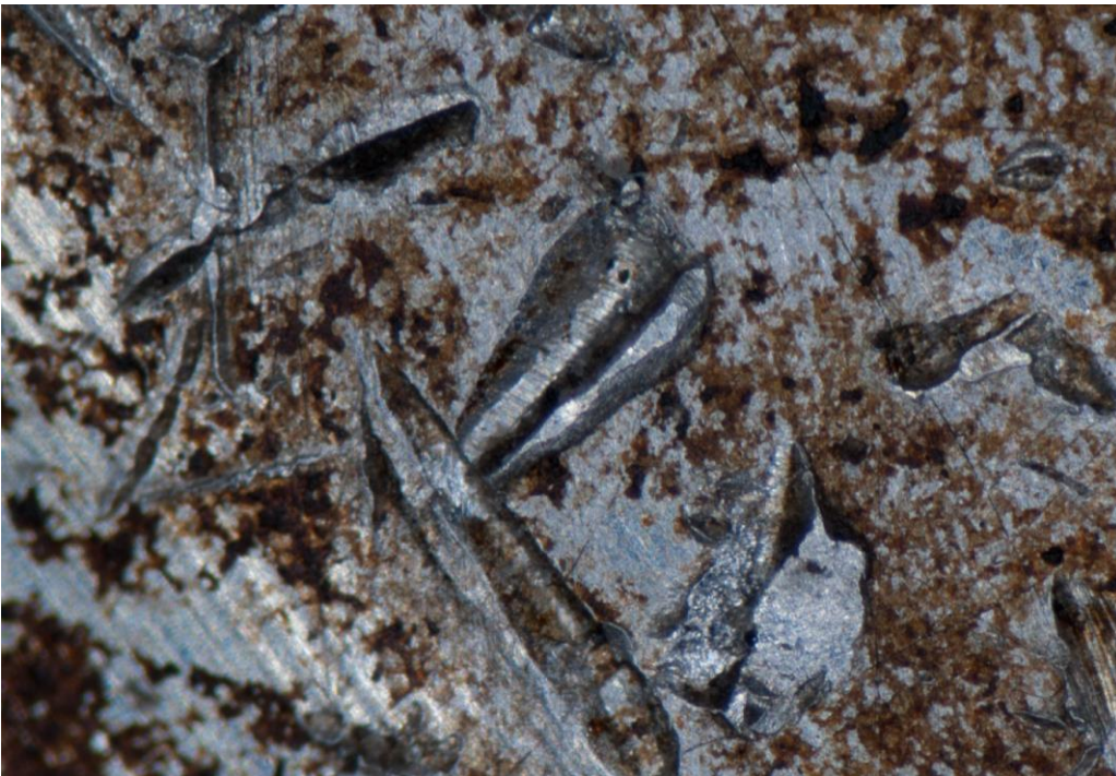
Figure 11: Damages on piston crown on piston no. 2. Photo: AIBN
