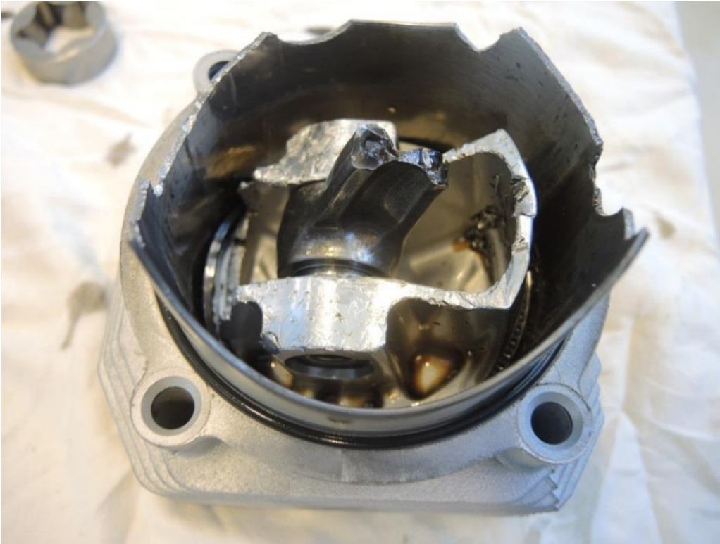
Figure 8: Cylinder no. 2 with piston and upper part of connecting rod. Photo: AIBN
