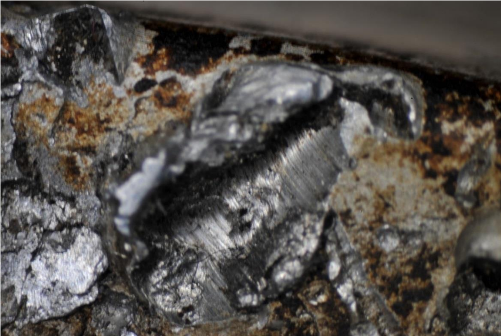
Figure 10: Traces of foreign objects on piston crown on piston no. 4. Photo: AIBN/NDLO
