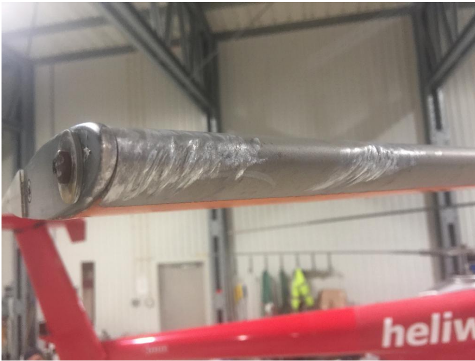
Figure 1: The damage to the tip of one of the rotor blades. Photo: Heliwest
