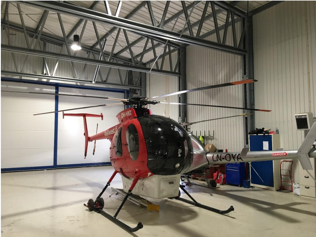
Figure 3: The helicopter photographed in the hangar at Gullknapp the day after the accident. The inspection equipment is mounted in the white pod under the belly of the helicopter. Photo: Agder Energi Nett
