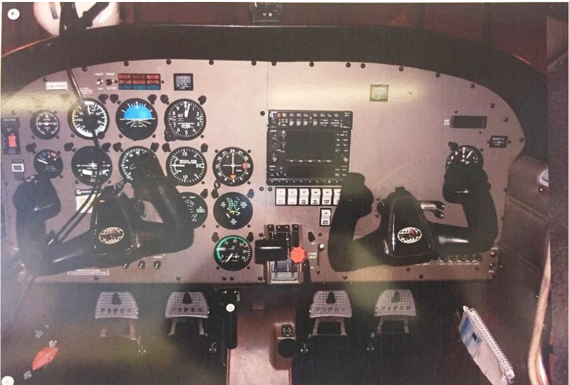
Figure 1: Instrument panel in LN-TOS. Six of the eight white switches in a row are visible in the centre of the image. Photo: Tromsø Flying Club
