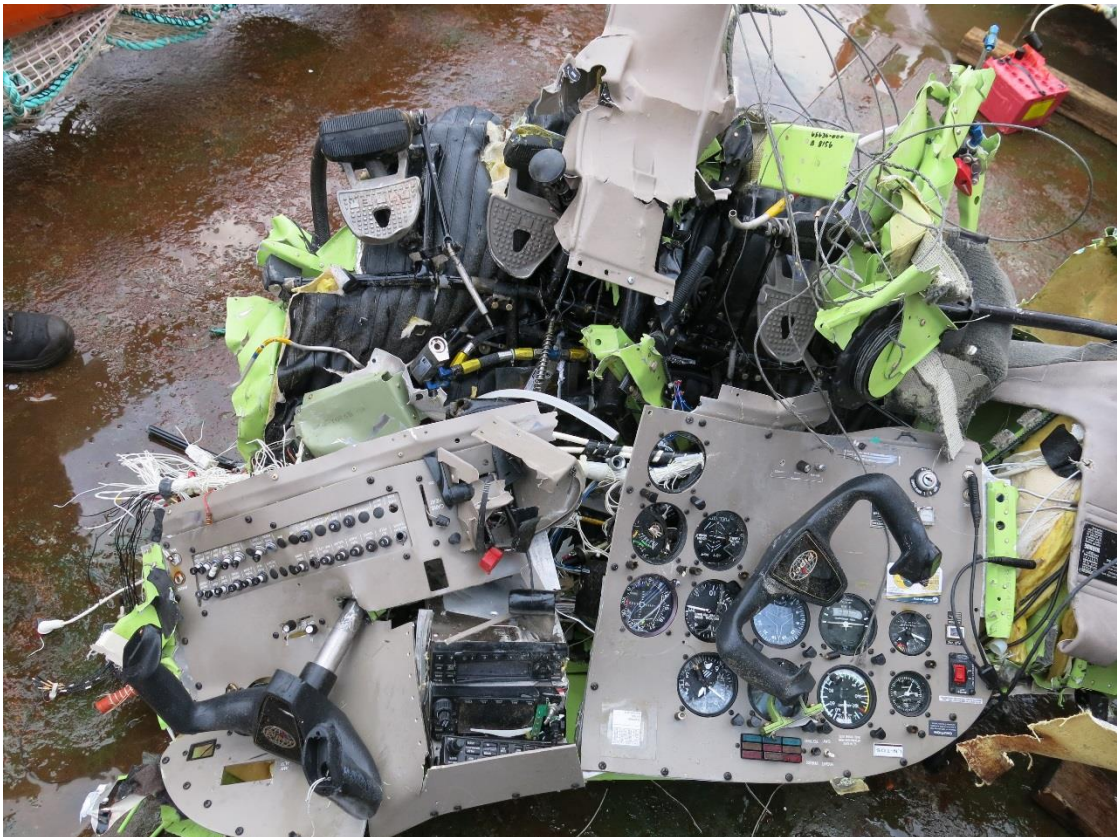
Figure 6: The instrument panel and flight controls after being raised from the seabed and placed on the recovery barge deck. Photo: AIBN
