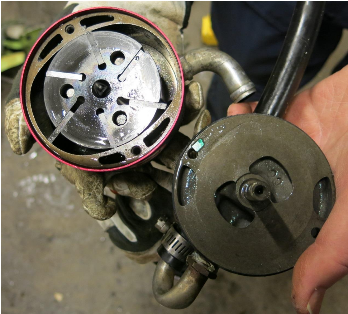
Figure 7: The vacuum pump after being opened up. Photo: AIBN
