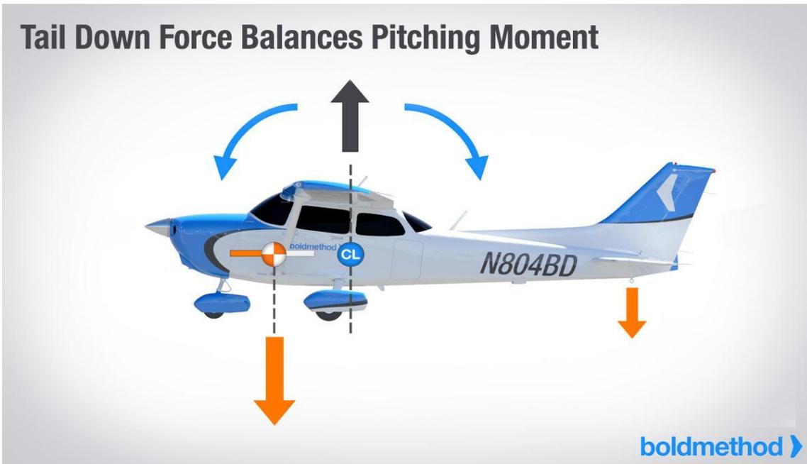
During cruise, ice isn't as big of a concern on the tail as it is on the wings. This is because the tail is usually at a low angle of attack and nowhere near performance limits. Any separated airflow around the tailplane stays relatively close to the ice buildup, allowing a majority of the effective airflow to remain attached around the tailplane and elevator. This changes and the greatest risk of a tailplane stall occurs when you increase flaps, or sometimes, power.
