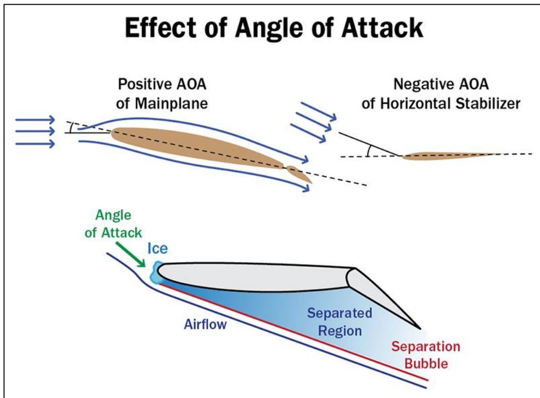
Figure 22: The effect of increased negative angle of attack on the tailplane. Source: "How to recover from Tailplane Icing" (Ross Detwiler)
