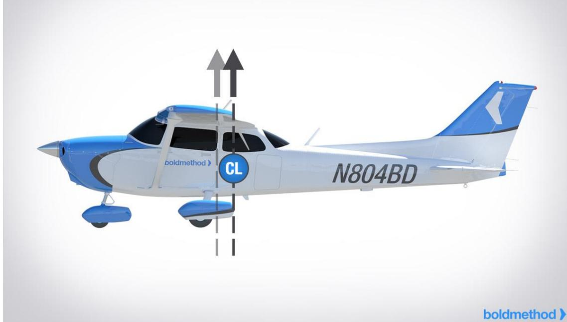
2) The tail's angle of attack increases due to the increased wing downwash.
