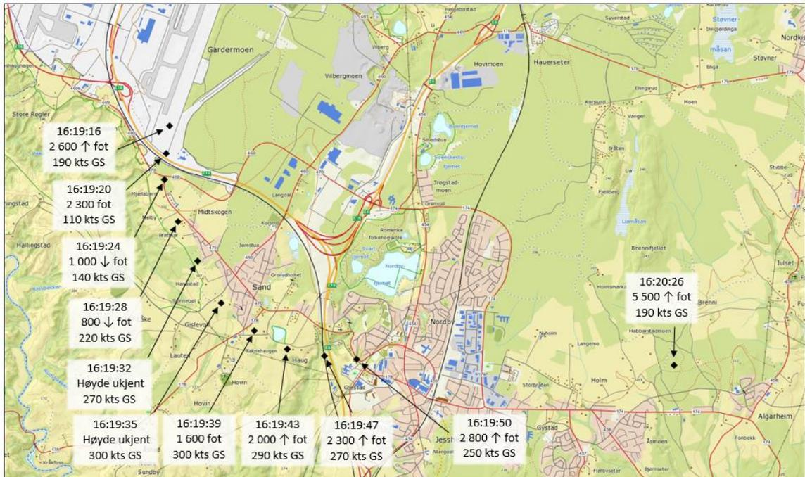
Figure 10: Estimated path of the flight based on radar data from Avinor. Map: © Norwegian Mapping Authority
