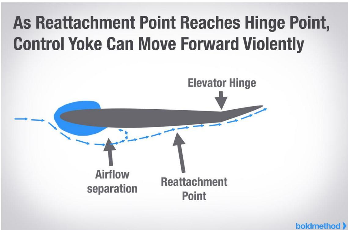
In short, large flap deflections, which produce large amounts of downwash, result in high angles of attack on the tailplane. With any ice accumulation on the leading edge of the horizontal stabilizer, increasing flaps, and sometimes power, will increase airflow separation around the tailplane. This is when you're most at risk for a tailplane stall.
