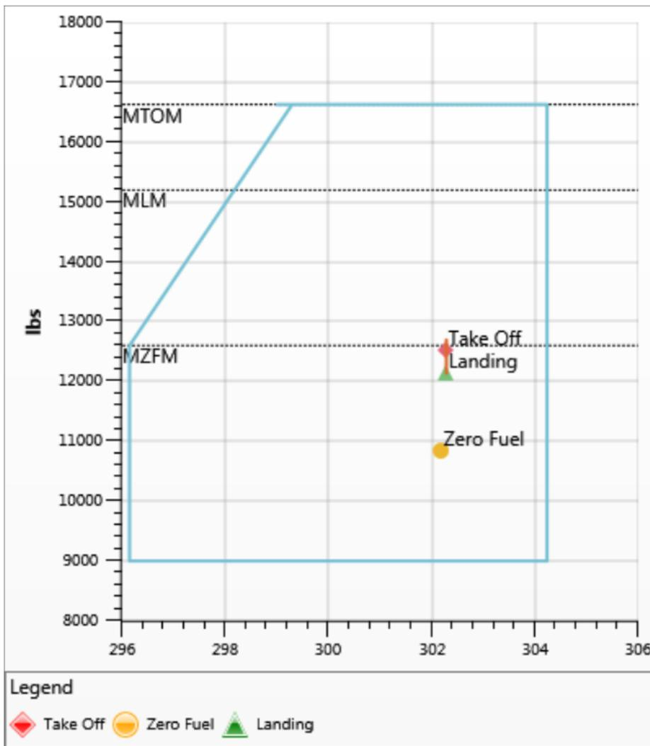
Figure 2: LN-IDB weight and balance diagram. Source: Hesnes Air AS
