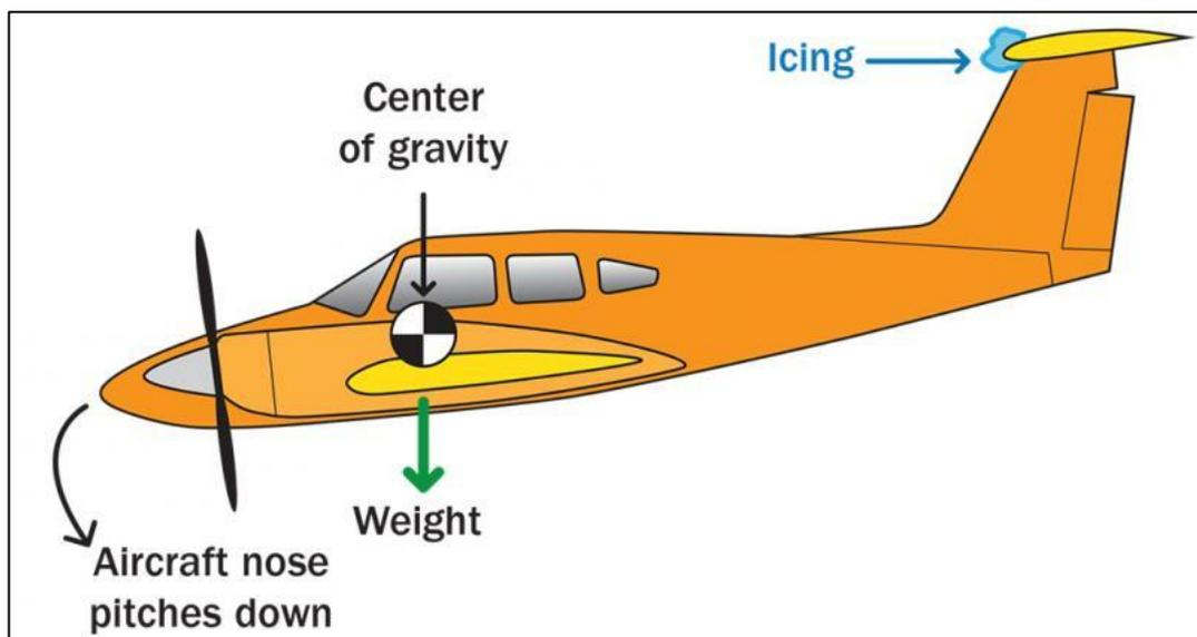
Figure 21: Tailplane stall as a result of icing. Source: "How to recover from Tailplane Icing" (Ross Detwiler)
