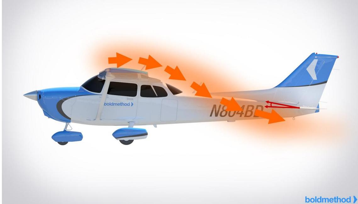
3) **More downward lift may be required** as the aircraft reaches equilibrium. This is accomplished by pulling back on the yoke and moving the elevator's trailing edge upward. Consequently the flap extension drives the horizontal stabilizer towards its critical angle of attack.
