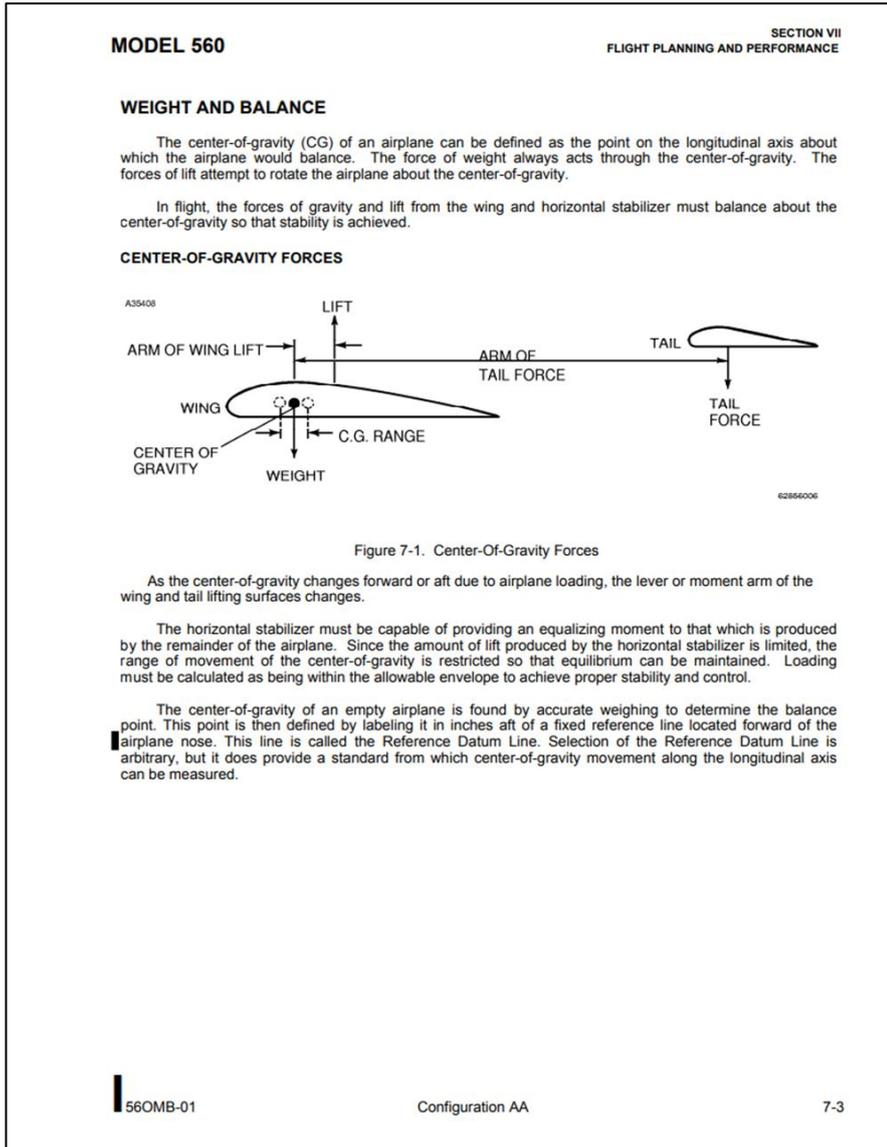
Figure 4: Note the negative lift on the tailplane. Source: Cessna FM Model 560
