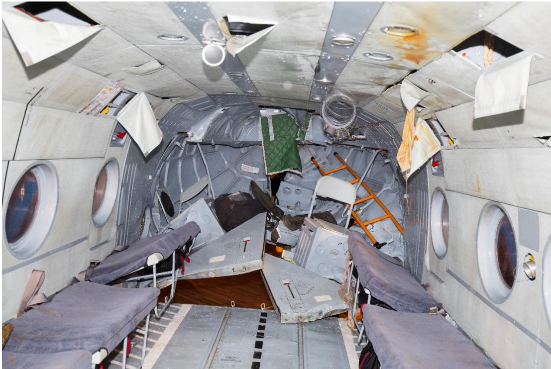
Figure 23: Deformed cargo doors due to impact with the water surface. The picture is taken looking towards the aft of the cabin and the cargo doors. Photo: The police
