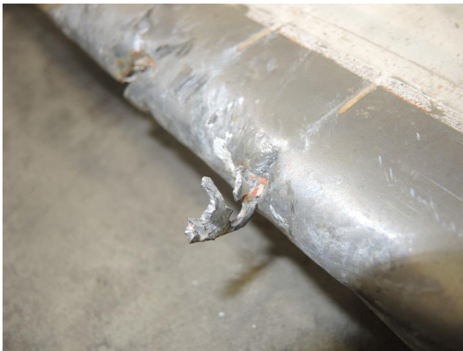
Figure 6: Fragment of FDR casing stuck in the leading edge of a main rotor blade. Photo: AIBN
