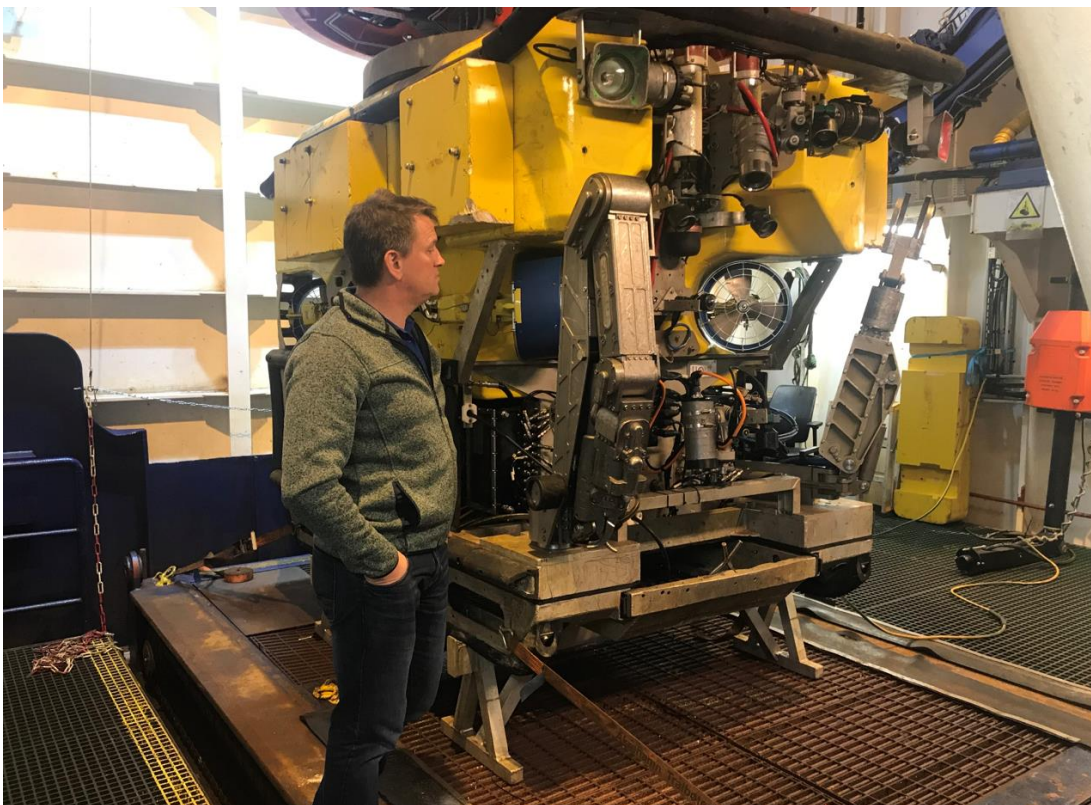
Figure 13: Maersk Forza ROV with manipulator arms. Photo: AIBN
