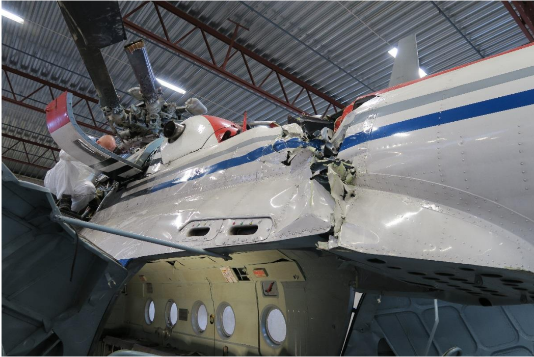
Figure 17: Structural damage on the left hand side between the main fuselage and the tail boom. Photo: AIBN
