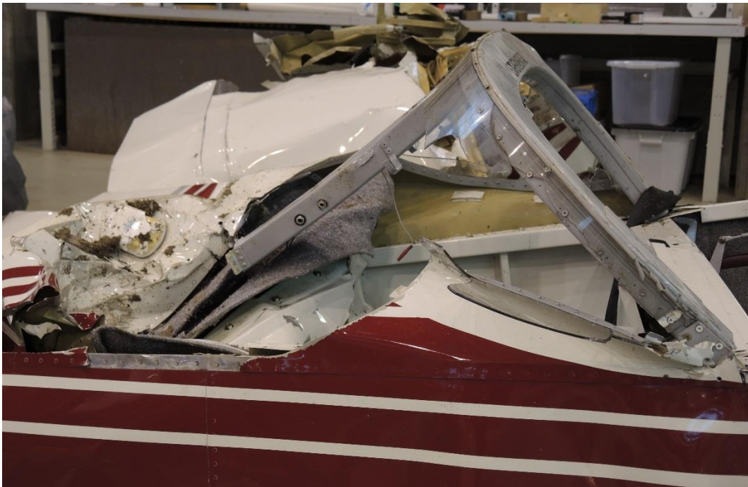
Figure 14: The frame in the canopy, which was bent all the way back and down (left). After the aircraft was turned over, the frame partially returned to its original position. Photo: AIBN
