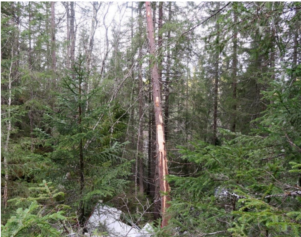
Figure 12: Photo taken facing north. The top of the photo shows the point of impact 9 meters up on the tree, which was tilted by the impact. The aircraft's right wing is visible to the left of the tree. Photo: AIBN
