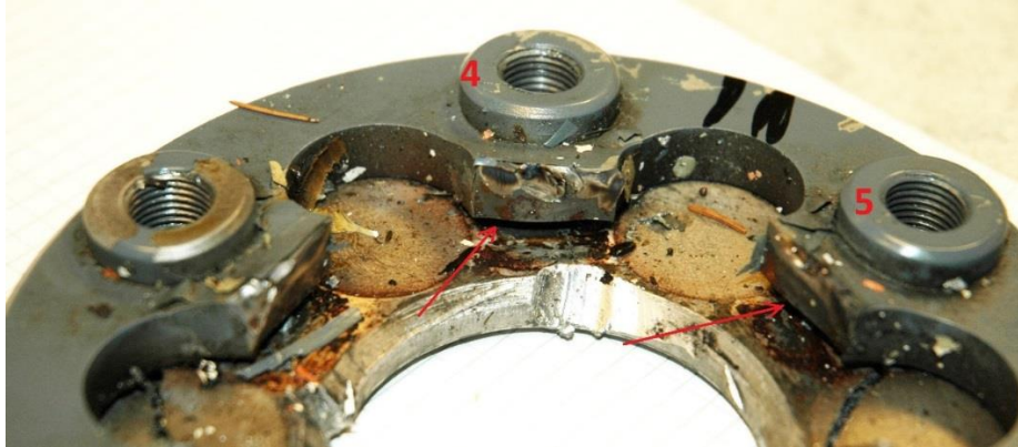
Figure 18: Parts of the propeller flange and parts of the disc that drives the generator belt and keeps the starter ring gear in place. The arrow shows the opening that formed as propeller bolts 4 and 5 were bent upwards. Photo: AIBN
