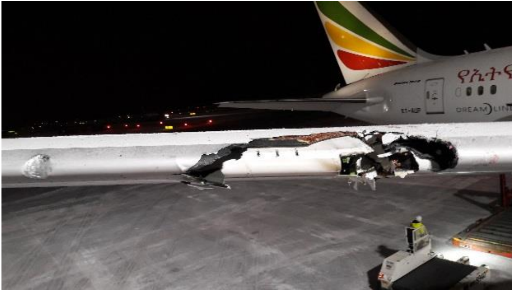
Figure 10: Damage to the right wing. Photo: Ethiopian aeronautical engineer
