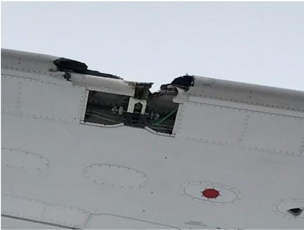
Figure 12: The damage. The surge tank can be seen in the background. Photo: AIBN
