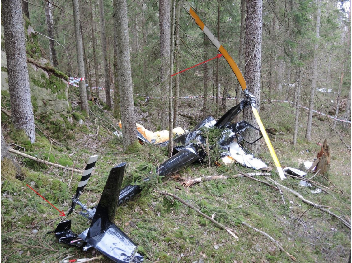
Figure 3: The accident site seen toward the northwest. The red arrows show a crack in one of the tail rotor blades and the bend in one of the main rotor blades. Photo: NSIA
