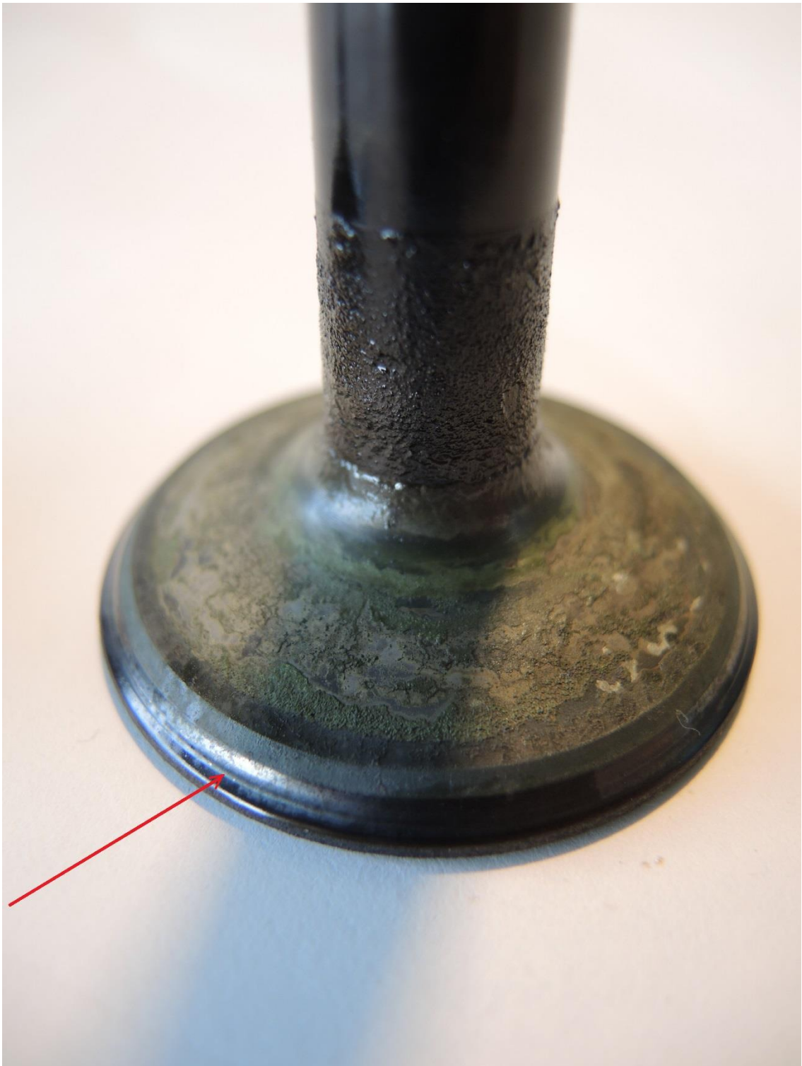
Figure 9: The exhaust valve from cylinder no. 5. The arrow points to the damage at the head face. The color of the valve is light brown with some green patches. Photo: NSIA
