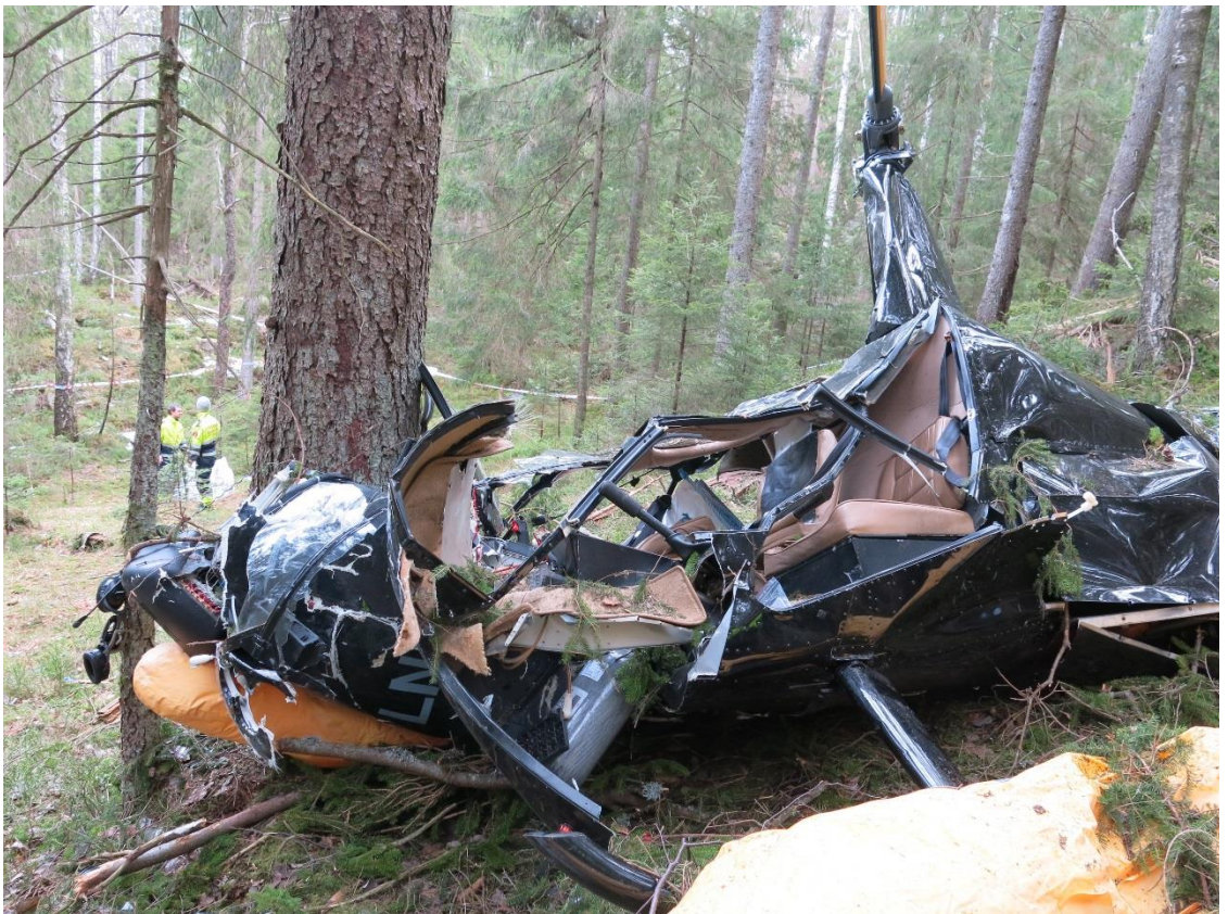
Figure 4: Damage to the cockpit/cabin. Photo: NSIA
