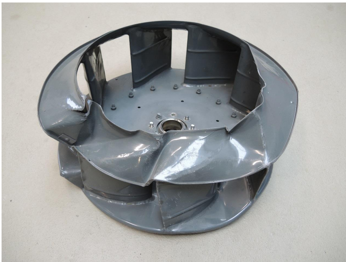
Figure 5: The underside of the engine's cooling fan was flattened. There was no visible sign that it had been rotating when it was damaged. Photo: NSIA
