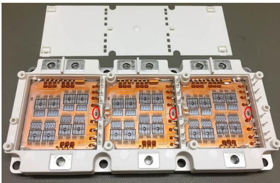
Figure 9: The three electronics chambers in the power controller. Three IGBTs with their associated temperature sensors indicated by a red circle. Illustration: EMSISO
