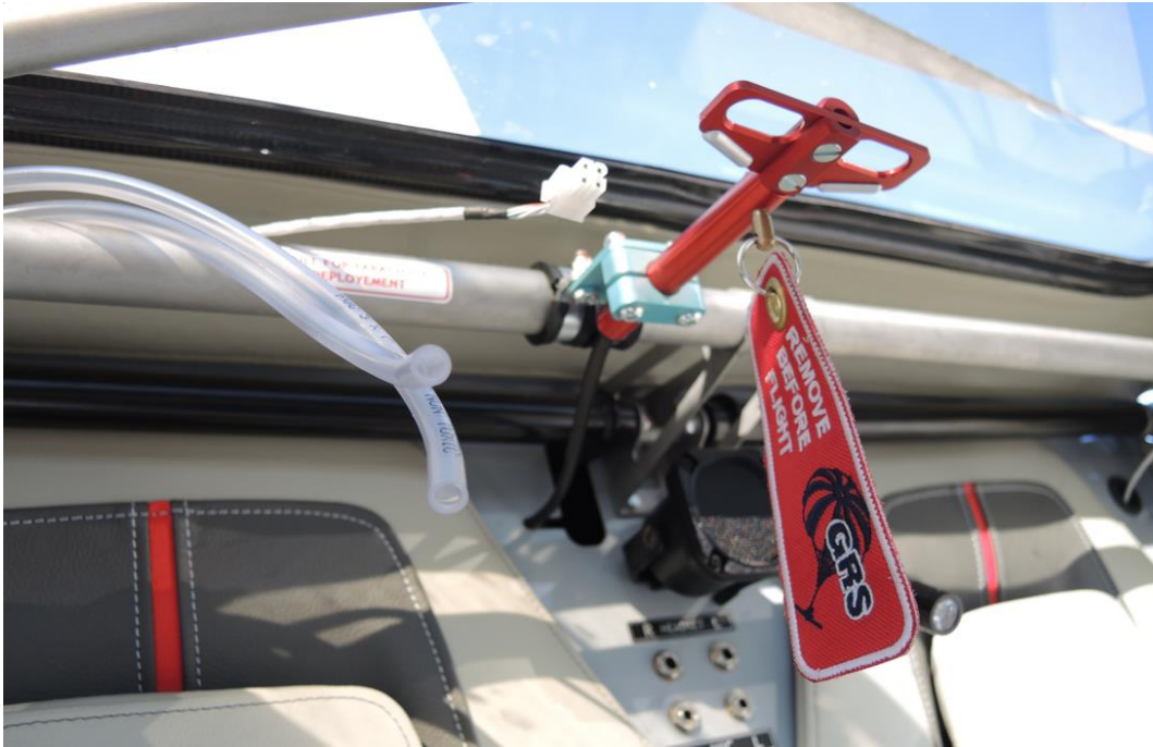
Figure 11: The emergency rescue parachute activation handle. Photo: NSIA
