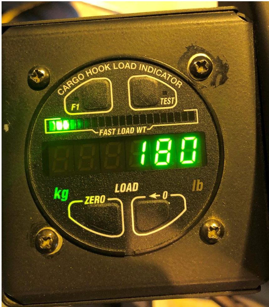
Figure 5: Two green diodes are lit to indicate a load of 180 kg. Reflections in the glass can give the impression that four diodes are lit. Photo: Helitrans AS
