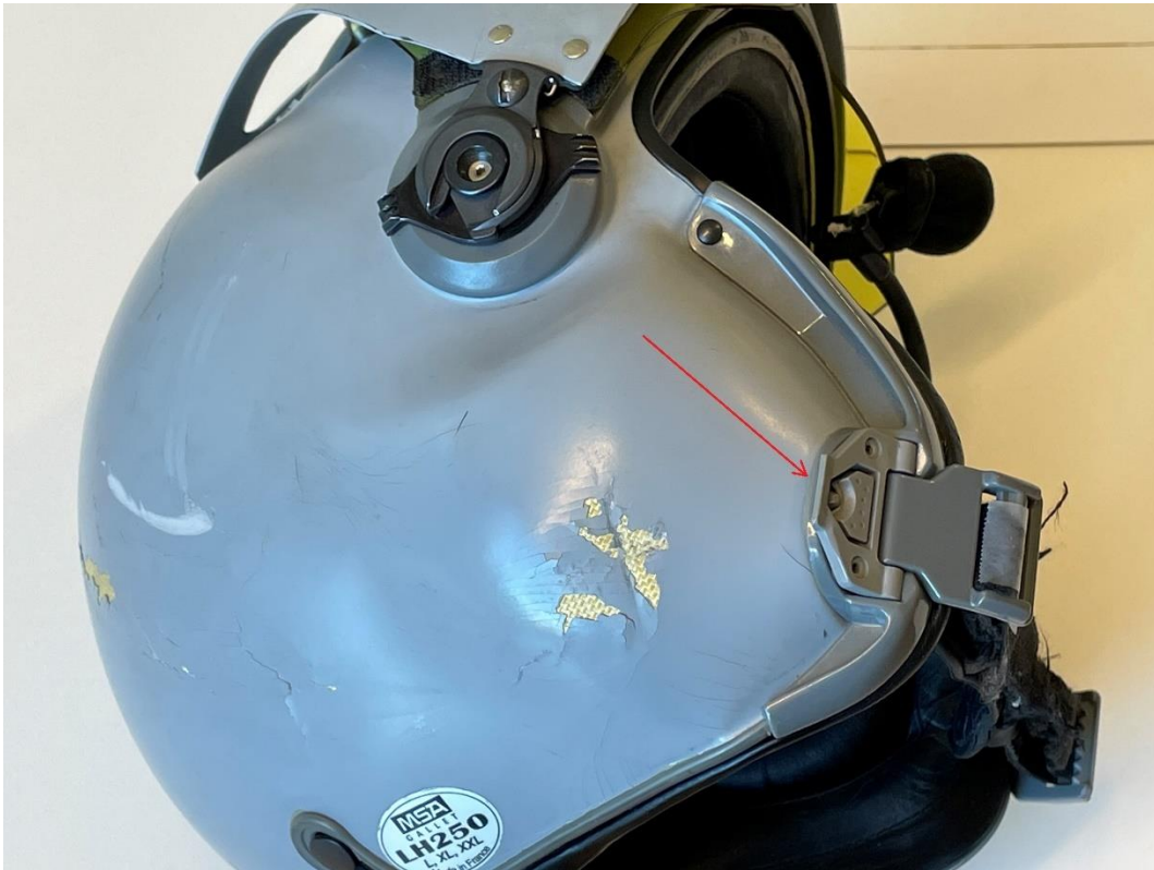
Figure 13: The commander's helmet, showing damage to the right side. The arrow points to the chin strap lock that came undone. Photo: NSIA
