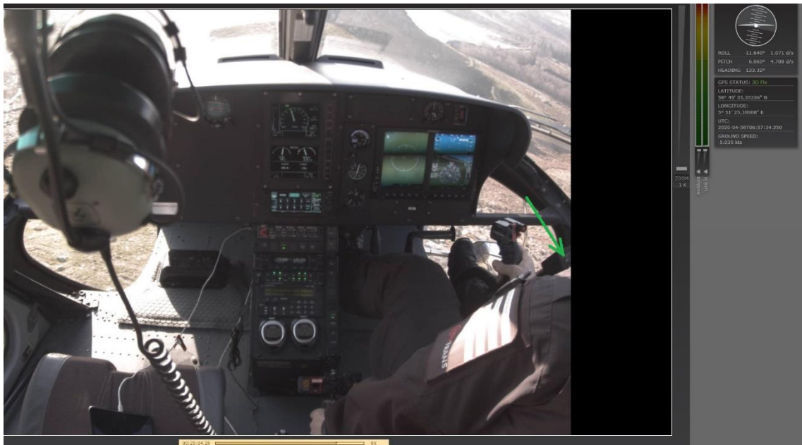
Figure 2: The helicopter has rolled left to an angle of 11.6 degrees and has a nose high angle of 6 degrees. The commander has moved the cyclic stick all the way to the right, and his right foot has just slipped off the pedal. A single green light can be seen on the far right in the image, indicating a load of less than 100 kg (green arrow). Source: Appareo Vision 1000/NSIA
