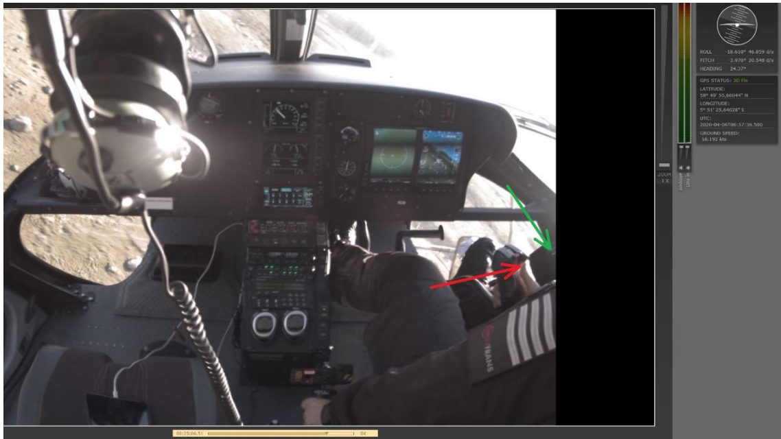
Figure 3: Two green lights (green arrow) can be seen on the far right in the image, indicating that the cargo hook load has exceeded 100 kg. The commander pressed the switch on the cyclic stick to release the cargo (red arrow). At this point in time, after spinning out of control, the helicopter had turned 116 degrees to the left. The nose angle had dropped to -4 degrees. Source: Appareo Vision 1000/NSIA
