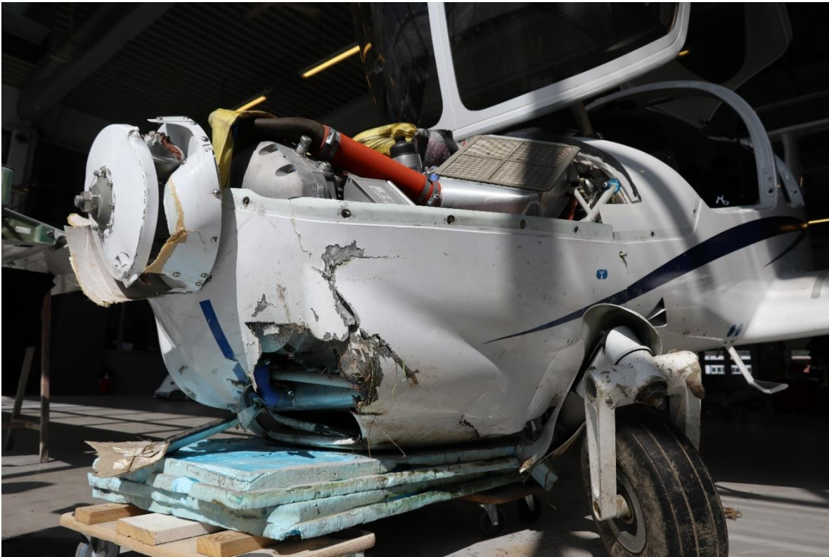
Figure 3: LN-PFJ photographed after it was moved to the hangar. The photo shows damage to the front of the fuselage, damaged landing gear and damaged propeller, where all the blades have been knocked off. Photo: NSIA
