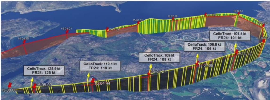
Figure 34: Comparison between data on ground speed and flight path from Flightradar24 (marked in yellow) and similar data from the CelloTrack unit (marked in red) carried by the helicopter on the accident flight. The comparison confirms the reliability of the signals. The accident site in the lower left corner is marked with a red pin and the time 15:08:00. Illustration: BEA/NSIA
