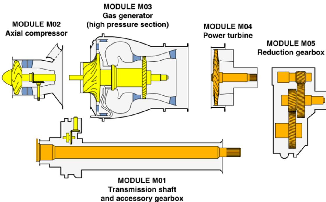
Figure 9: The five main modules of SHE's Arriel 2D engine. Illustration: Safran Helicopter Engines/NSIA
