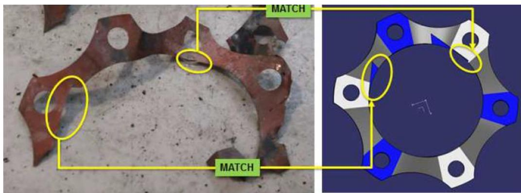
Figure 55: Comparing the damages to the actual disc segments of LN-OFU and typical damages to the disc segments due to misalignment of the driveshaft it was found that they were close to identical. Source: Airbus Helicopters/NSIA
