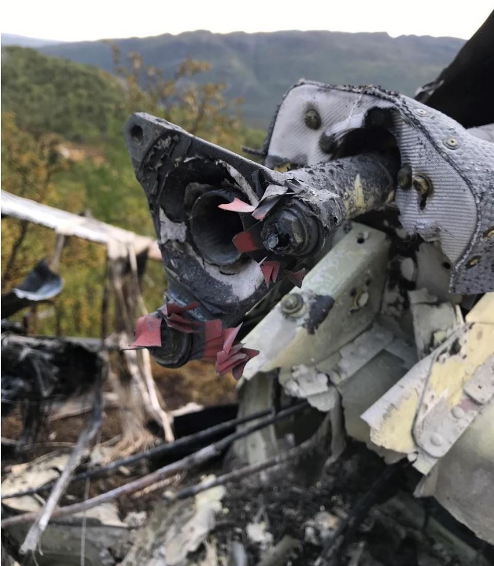
Figure 29: The broken drive shaft for the tail rotor between the fuselage and tail boom, with typical rupturing of the flexible coupling. Photo: NSIA
