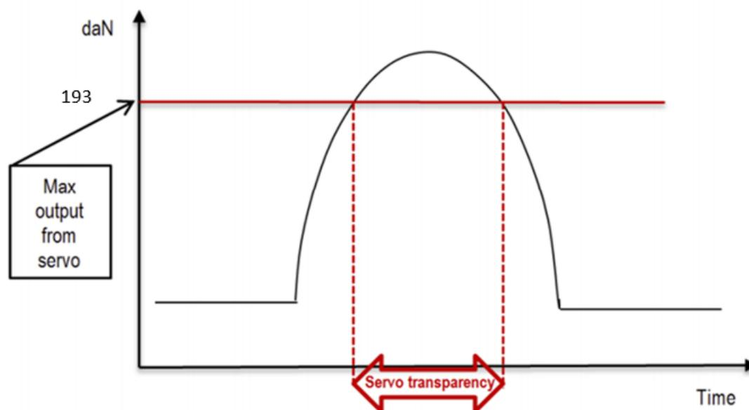
Figure 18: Illustration of servo transparency. The output needed exceeds the capacity of the servo actuators for the period between the red dashed lines. Illustration: NSIA
