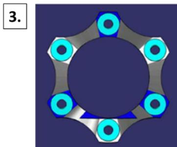
Figure 54: The illustration from the animation shows how the damages to the flexible coupling discs can be created after contact with the drive shaft due to misalignment between engine and main gear box. Source: Airbus Helicopters/NSIA
