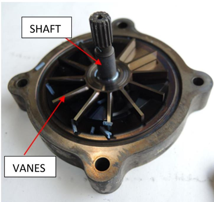
Figure 62: The vanes and shaft in the low-pressure part of the fuel pump. Small bits of the interior blue gasket were further fragmented and fell off during disassembly. Photo: NSIA
