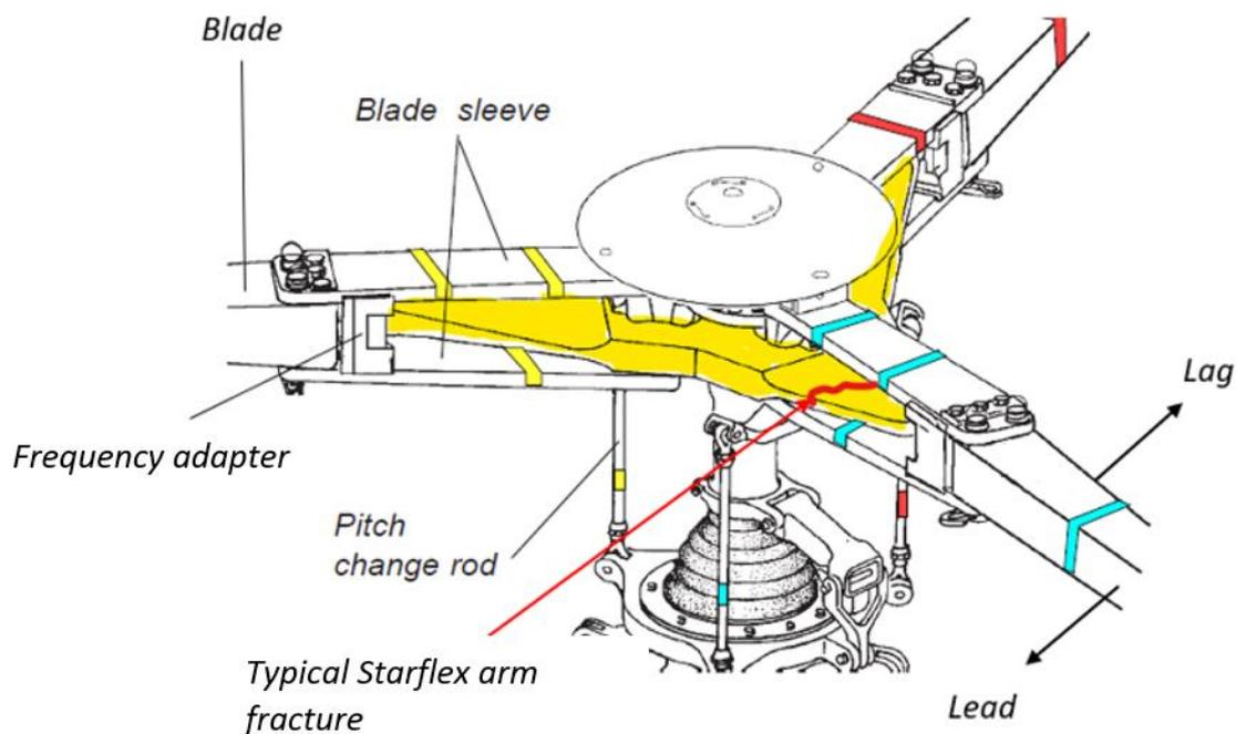
Figure 16: The Starflex hub with Starflex arms are marked in yellow. The arms will typically fracture as indicated in red. The fracture can also go in the opposite direction. Illustration: Airbus Helicopters/NSIA
