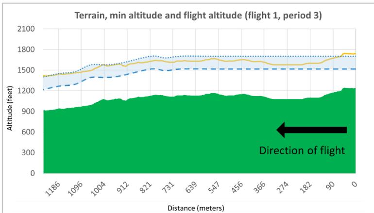
Figure 41: Altitude above the terrain during the last period of the first sightseeing flight. The green represents the terrain, the amber line shows the minimum altitude of 500 ft above the terrain, while altitude of the flight path is indicated in blue. The upper blue dotted line represents altitude data from Flightradar24, and the lower dotted line is the altitude of the flight path adjusted with data from CelloTrack. Source: NSIA
