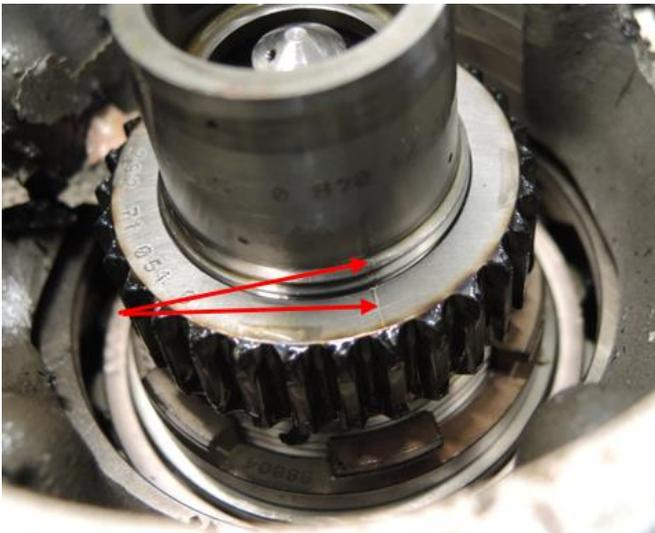
Figure 67: The alignment marks on LN-OFU. The blue discoloration of the nut was caused by the heat that developed after the crash. Photo: Safran Helicopter Engines/NSIA
