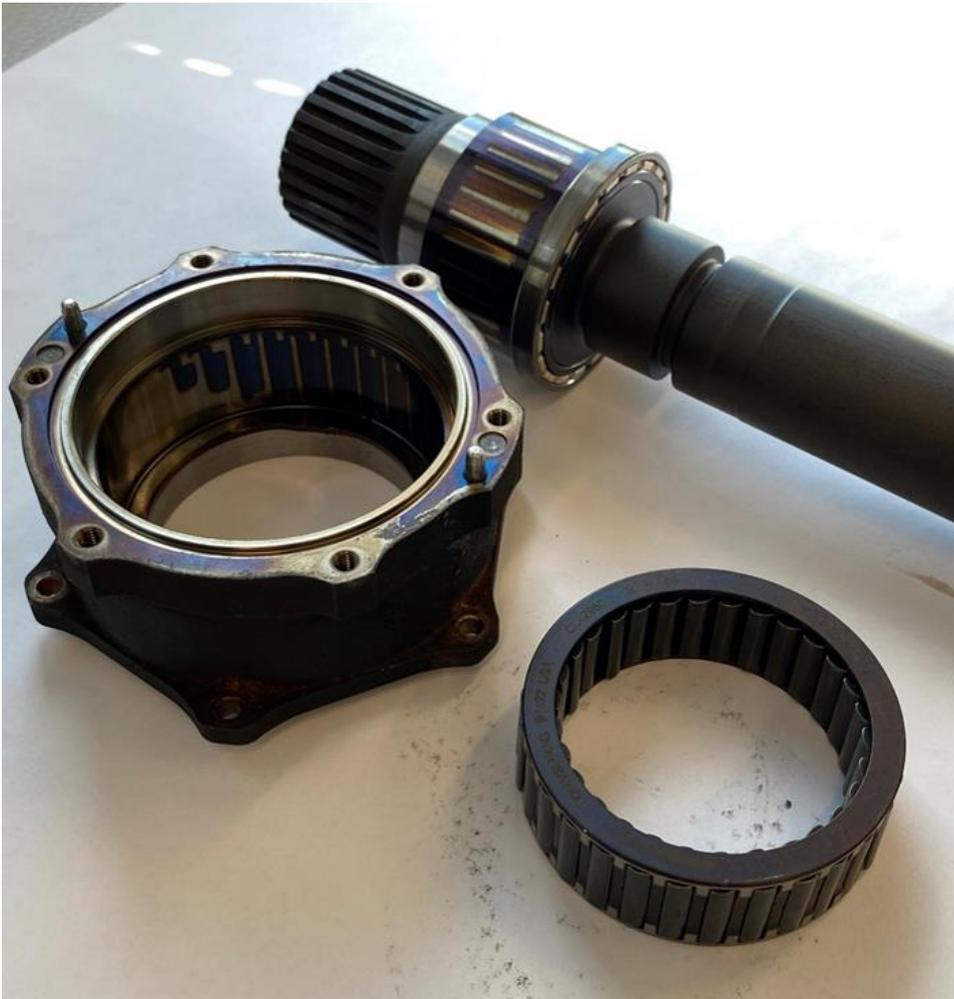
Figure 66: The freewheel clutch. From left to right: the outer ring with blue oxidation marks, the inner shaft with oxidation marks from the sprags and the ring with sprags on the bottom right. Photo: NSIA
