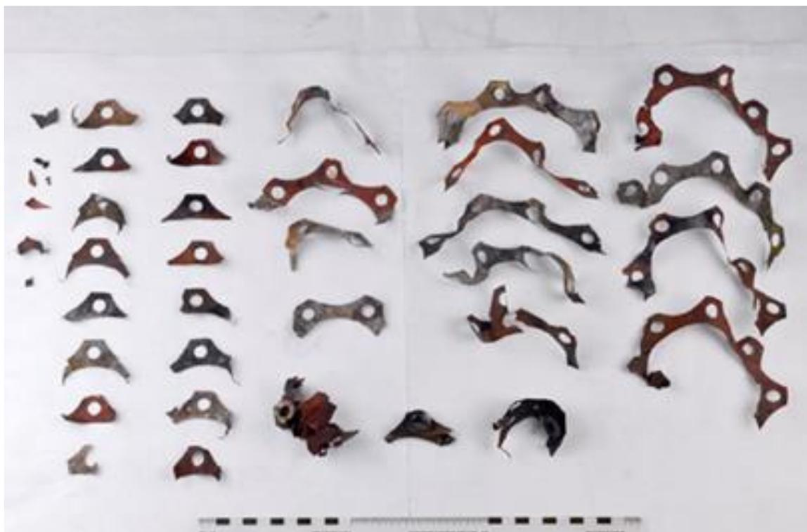
Figure 53: Disc segments from the flexible coupling. Photo: DNV GL and NSIA
