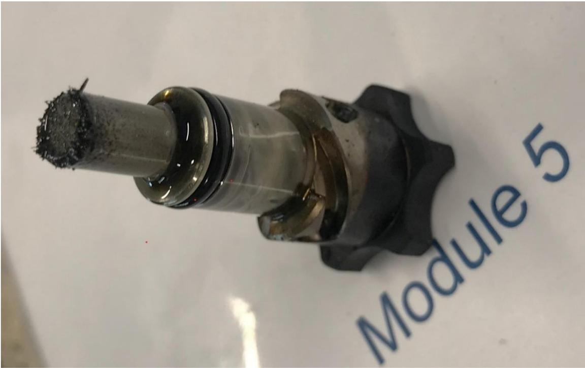
Figure 57: Magnetic oil plug in Module M05. Photo: NSIA
