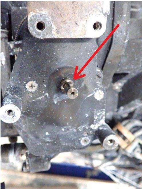
Figure 61: The arrow points to the locking finger on the shaft between the HMU and the EBCAU. When it points straight upwards, the EBCAU has not taken over control of the engine. Photo: Safran Helicopter Engines
