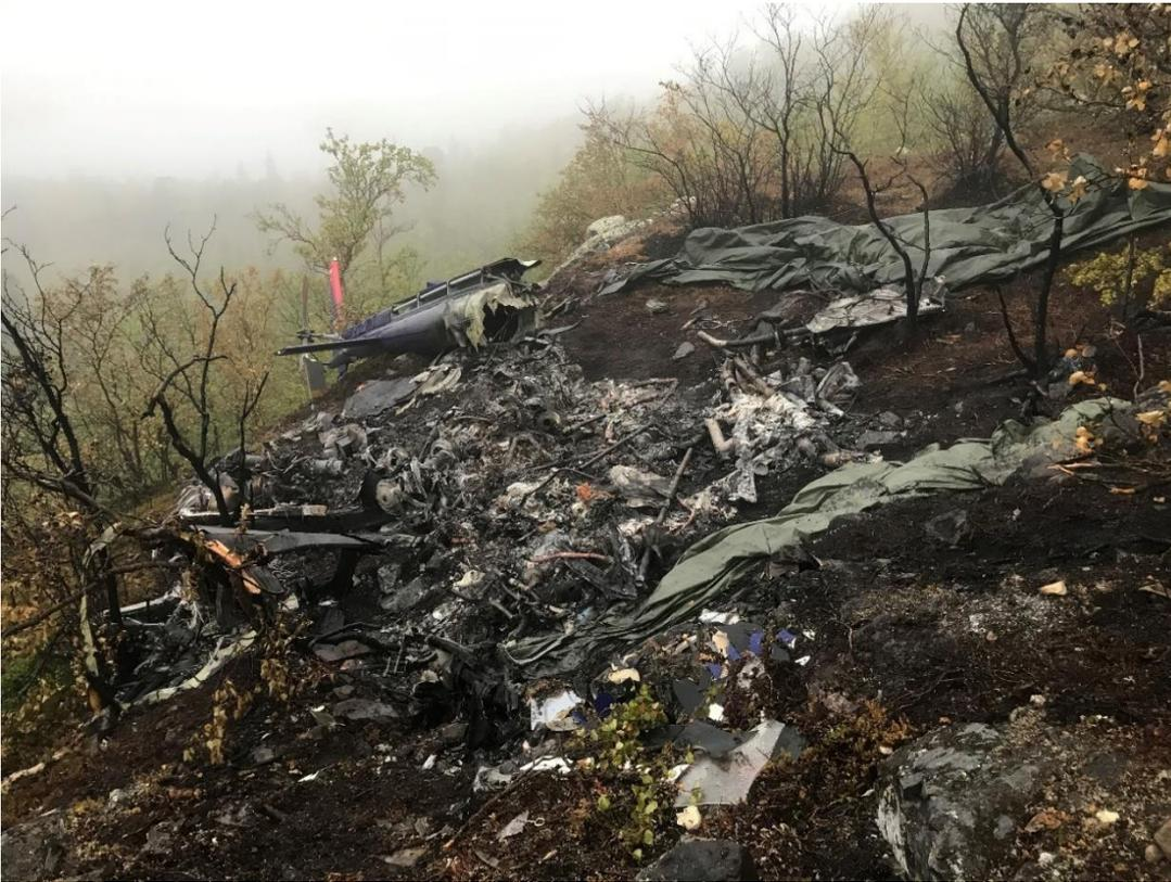
*Figure 25: The accident site near Skoddevarre, viewed from an easterly direction, with the front of the helicopter in the foreground. The bushes on the far right in the photo had not been damaged by the main rotor. Tarpaulins have been deployed to protect the wreckage. The photo was taken after removal of the deceased. Photo: NSIA*
