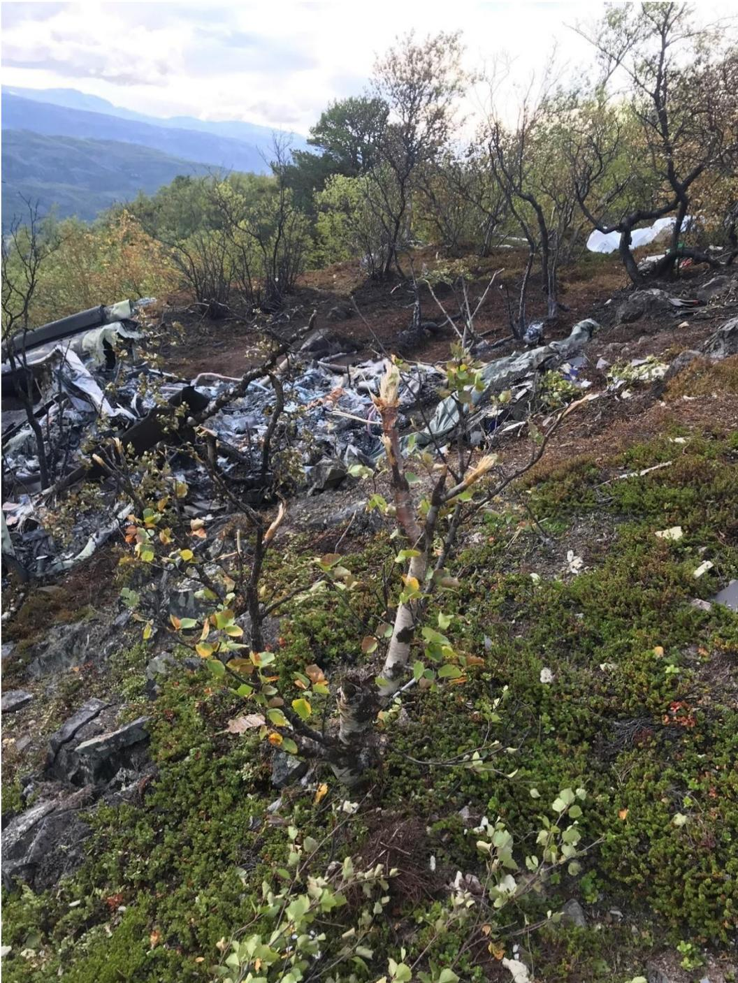
*Figure 26: The accident site, viewed from the south-east. The birch in the foreground was in front of and to the right of the wreckage. The tree on the upper right was damaged by fire only. Photo: NSIA*
