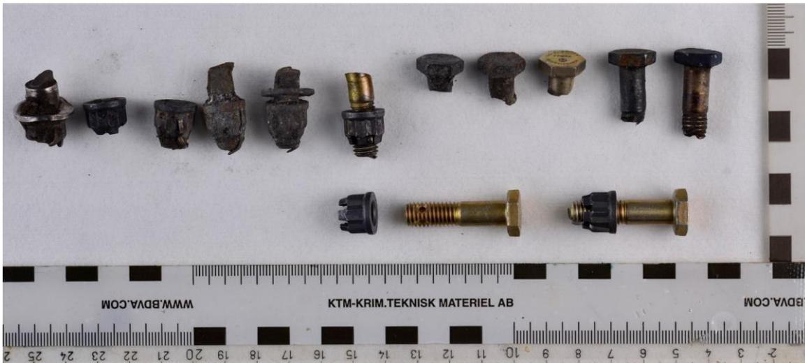
Figure 50: All the bolt halves that were found. For reference purposes, two unbroken bolts with nuts are shown in the lower part of the photo. Photo: DNV GL/NSIA
