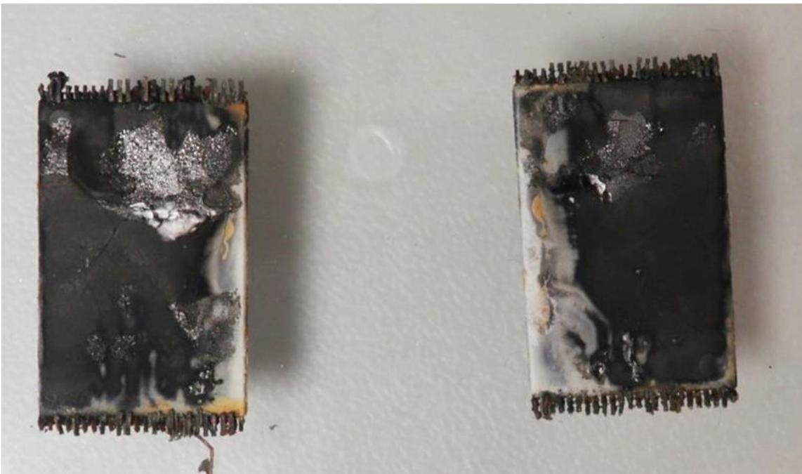
Figure 22: The memory units from the Appareo unit examined by Thales. Photo: BEA
