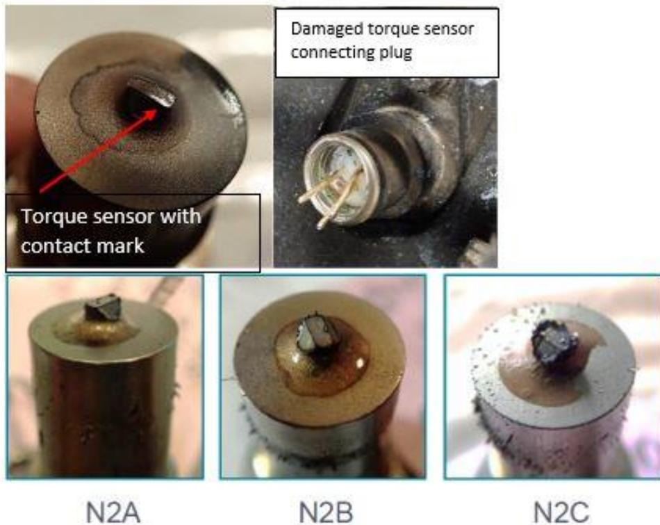
Figure 64: The torque sensor with contact mark on the pick-up part, the damaged connecting plug and the three undamaged N2 sensors. Photo: Safran Helicopter Engines/NSIA
