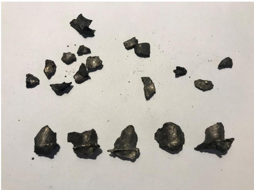
Figure 60: Turbine blade fragments found during engine disassembly. Photo: NSIA
