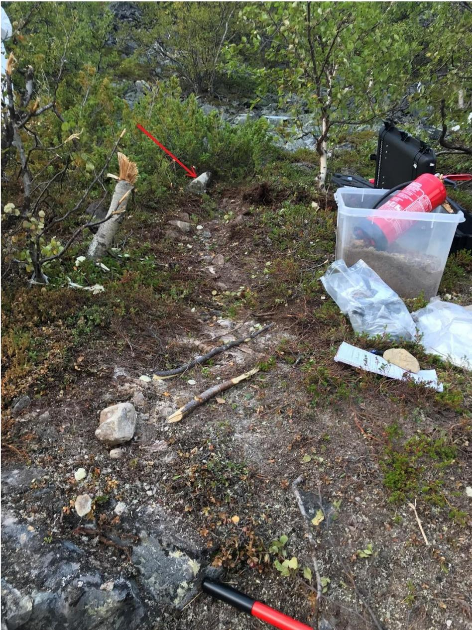
Figure 27: Photograph showing the most visible mark after a rotor blade to the front and to the left of the wreckage. The birches to the left in the photo have been cut by rotor blades. The red arrow shows where the tip of a rotor blade has hit a rock. Photo: NSIA
