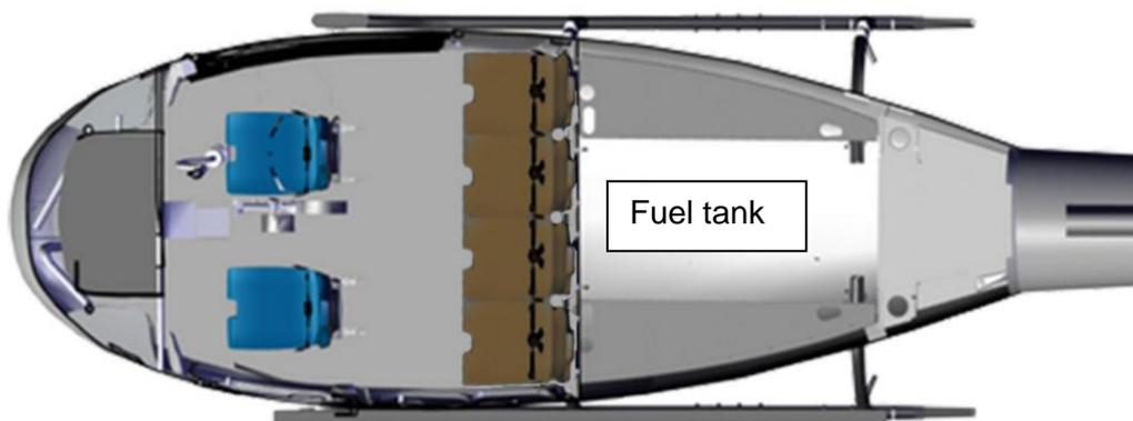
Figure 6: Position of seats and fuel tank in helicopter. Source: Airbus Helicopters/NSIA
