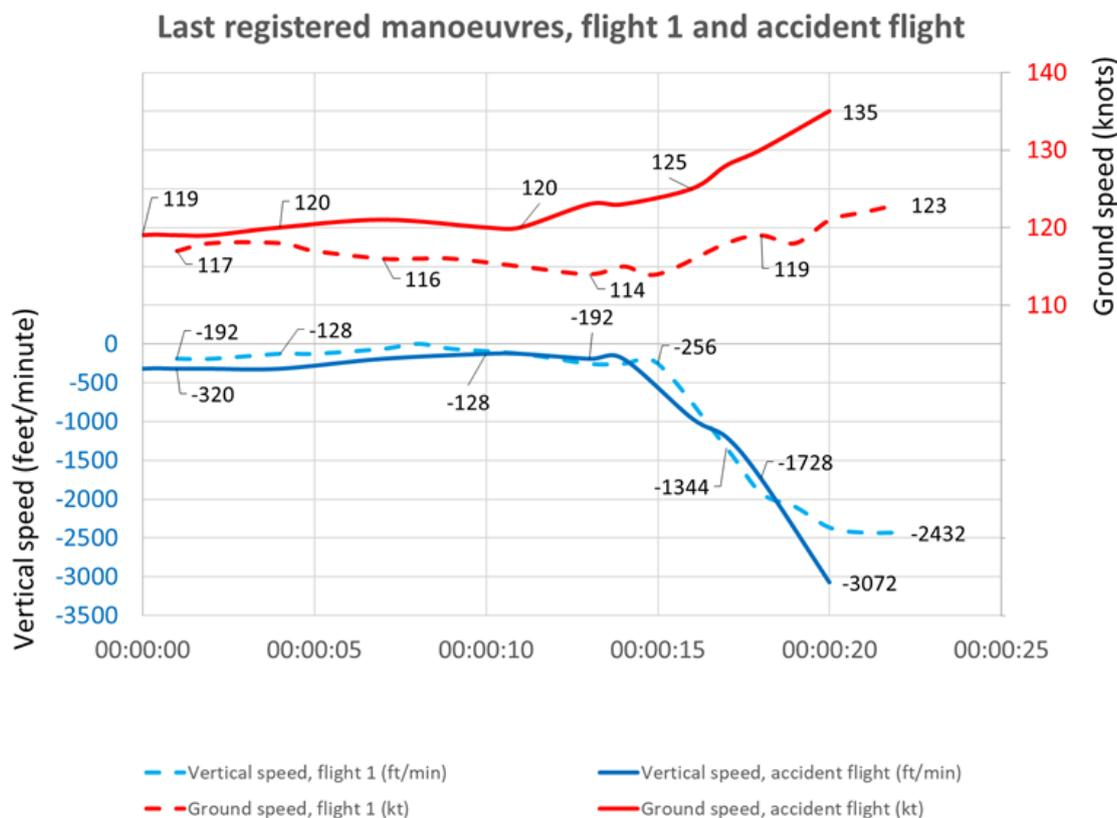
Figure 71: Last helicopter movements registered by FlightRadar24. Comparison between the last recorded manoeuvre (approx. 20 seconds) on the first sightseeing flight and the accident flight. Source: NSIA
