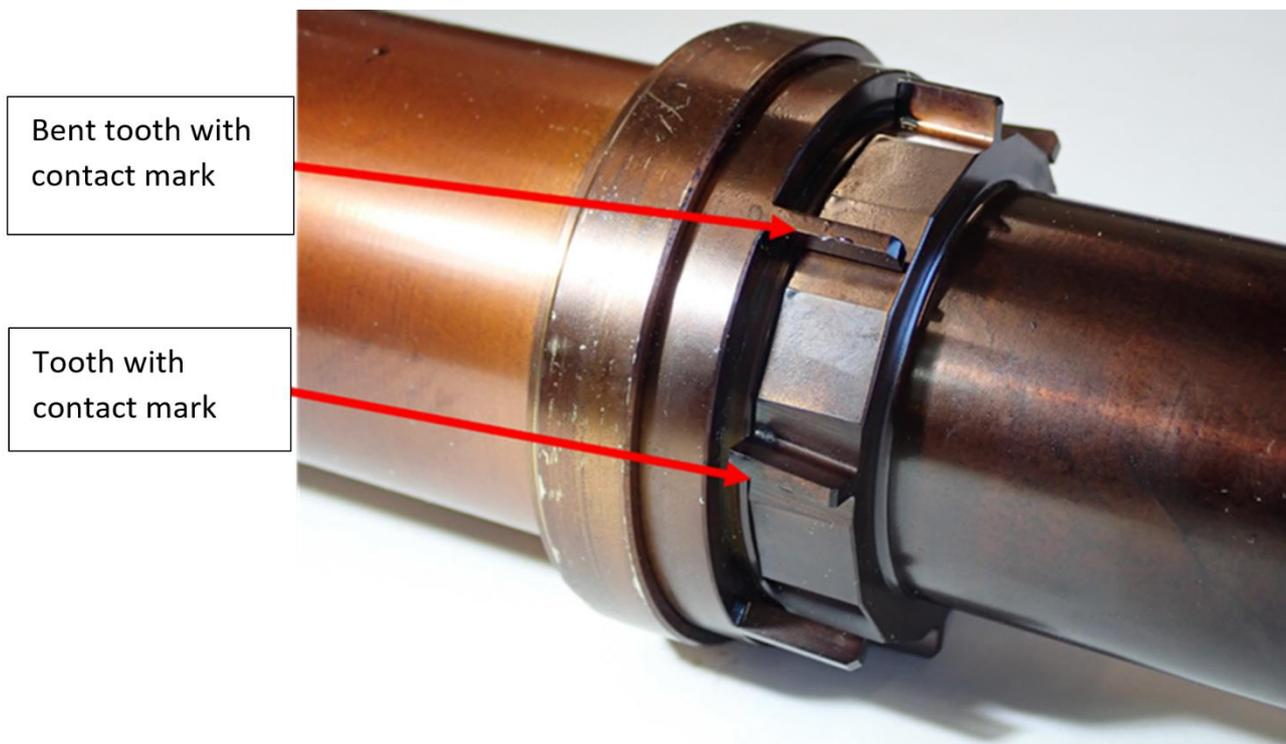
Figure 65: The engine's transmission shaft with contact mark and bent tooth. Photo: NSIA
