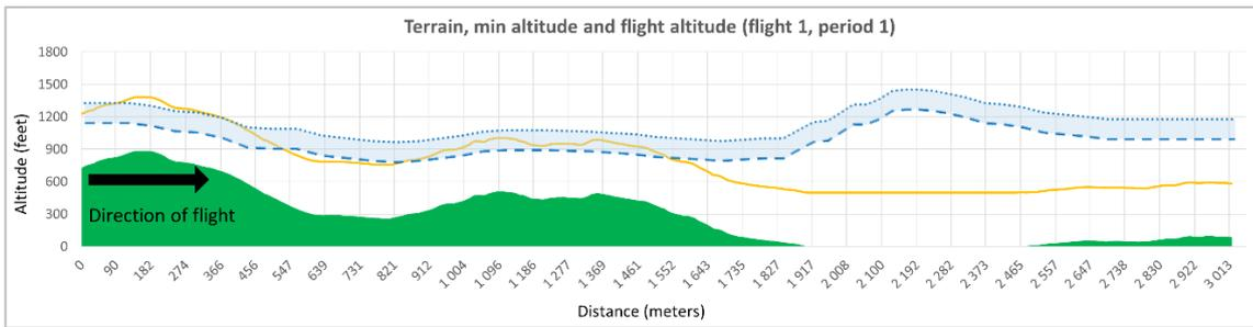
Figure 39: Altitude above the terrain during the first period of the first sightseeing flight. The green represents the terrain, the amber line shows the minimum altitude of 500 ft above the terrain, while altitude of the flight path is indicated in blue. The upper blue dotted line represents altitude data from Flightradar24, and the lower dotted line is the altitude of the flight path adjusted with data from CelloTrack. Note that the direction of flight is from right to left. Source: NSIA
