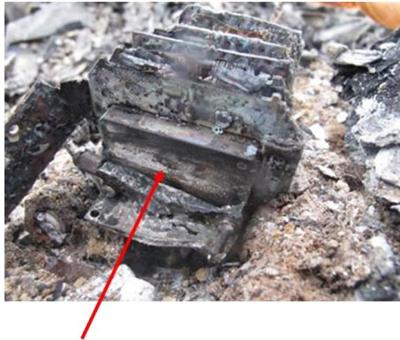
Figure 21: Appareo Vision 1000 in undamaged condition, and in severely fire-damaged condition as found in LN-OFU. The arrow points to the casing around the built-in memory module. Source: Appareo Systems, LLC and Airbus Helicopters
