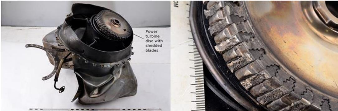
Figure 59: All 37 blades on the free turbine had just about identical fracture surfaces at the root of the blade. Photo: DNV GL/NSIA
