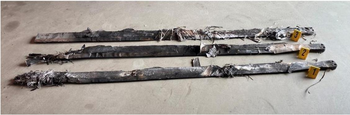
Figure 28: The three rotor blades. The blade tips are to the left in the photo. Photo: NSIA
