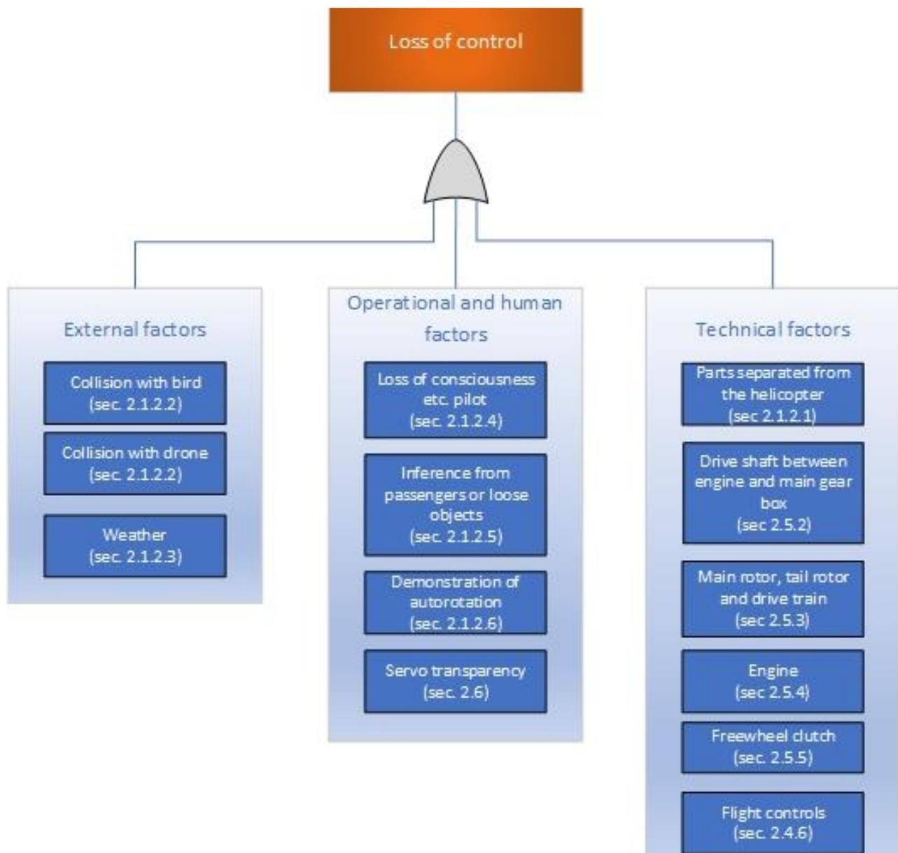
Figure 70: Simplified fault tree model – scenarios that could lead to loss of control, followed by impact with the ground and fire. Reference to section in the analysis. Illustration: NSIA
