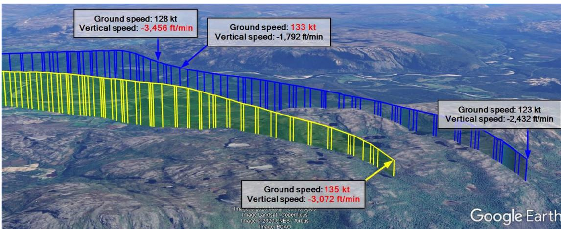
Figure 5: Comparison between the final part of the first flight and the final part of the accident flight. The first flight is indicated in blue while the accident flight is indicated in yellow. The values highlighted in red are the highest values. Source: Google Earth/BEA/NSIA
