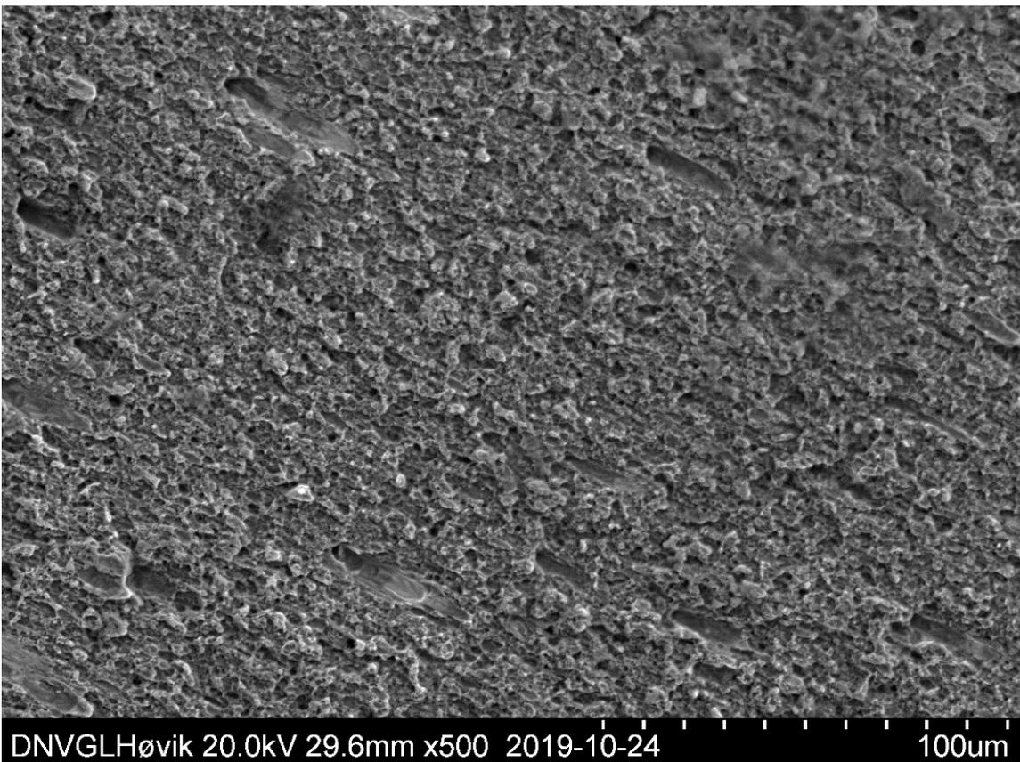
Figure 52: The fracture surface of the bolt in the previous figure, magnified 500 times. The dimples in the fracture surface are evidence of a ductile overload fracture. Photo: DNV GL/NSIA
