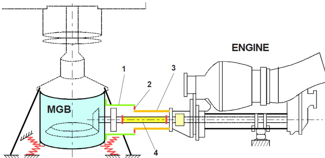
Figure 14: Connection between engine and main gearbox. Illustration: Airbus Helicopters/NSIA
