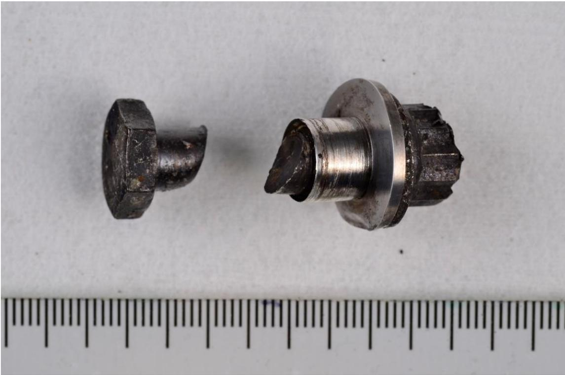
Figure 51: The fracture surfaces of one of the bolts. The sleeve that is inserted through the discs can be seen on the right by the nut. Photo: DNV GL/NSIA
