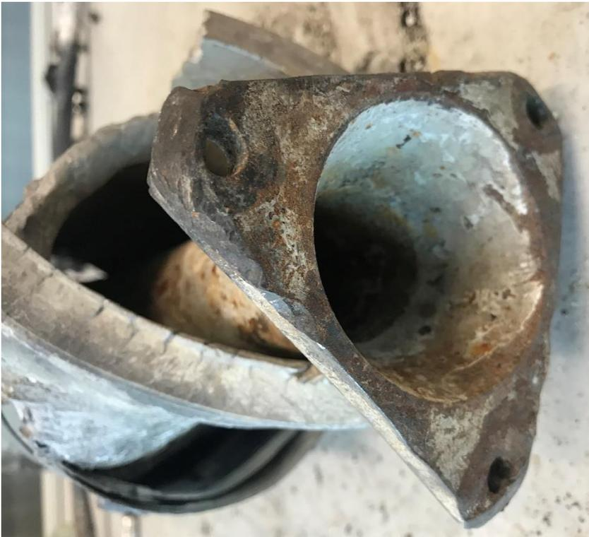
*Figure 49: Drive shaft between engine and main gearbox with flange for connection to the gearbox. The flange shows rotation damage in several places and no remains of the flexible coupling. The gimbal coupling in the background is severely damaged by heat and also shows signs of rotation damage. Photo: NSIA*
