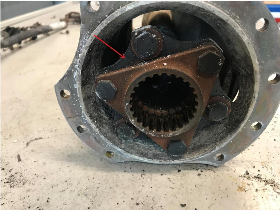
Figure 48: The drive shaft between the engine and main gearbox seen from the engine side. The flexible coupling, see red arrow, appears to be undamaged. Photo: NSIA
