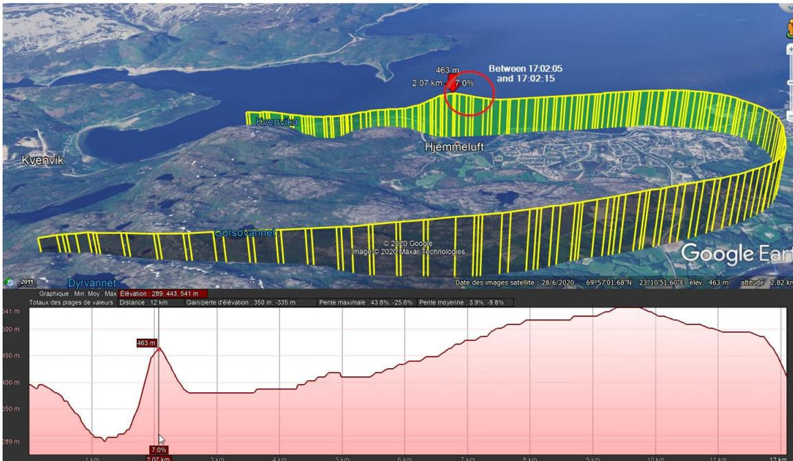
Figure 4: Vertical profile of flight path at the time when the photo above Hjemmeluftbukta was taken. The graph shows the helicopter's altitude above ground level. Illustration: Flightradar24/BEA/NSIA
