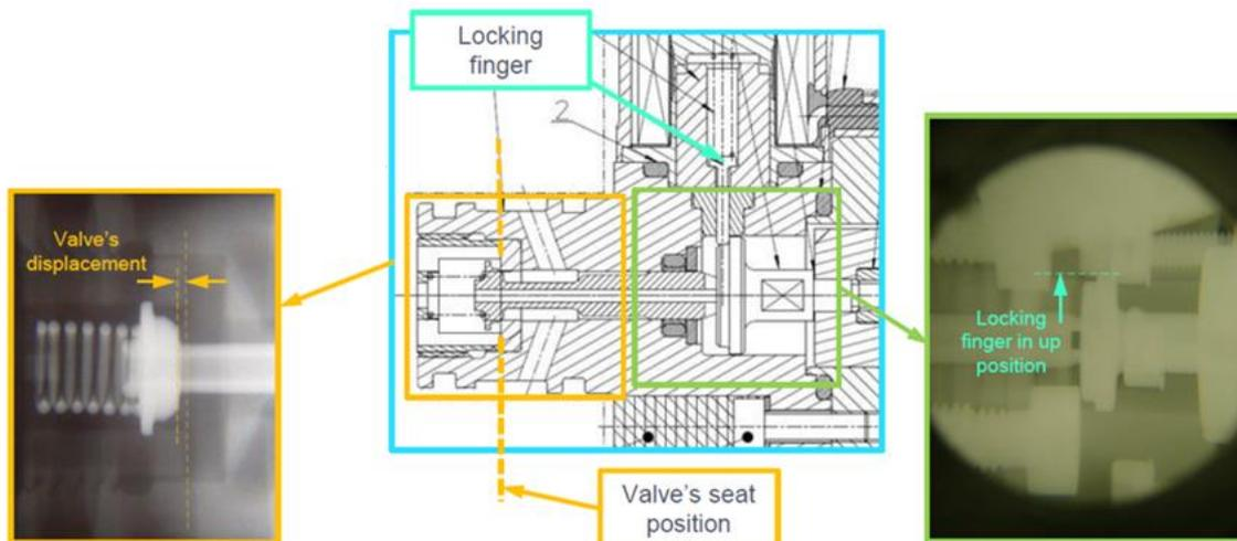
Figure 63: X-ray images of the SEV showed that it was found in the open position and had not been activated. Illustration: Safran Helicopter Engines. X-ray images: AIM/NSIA
