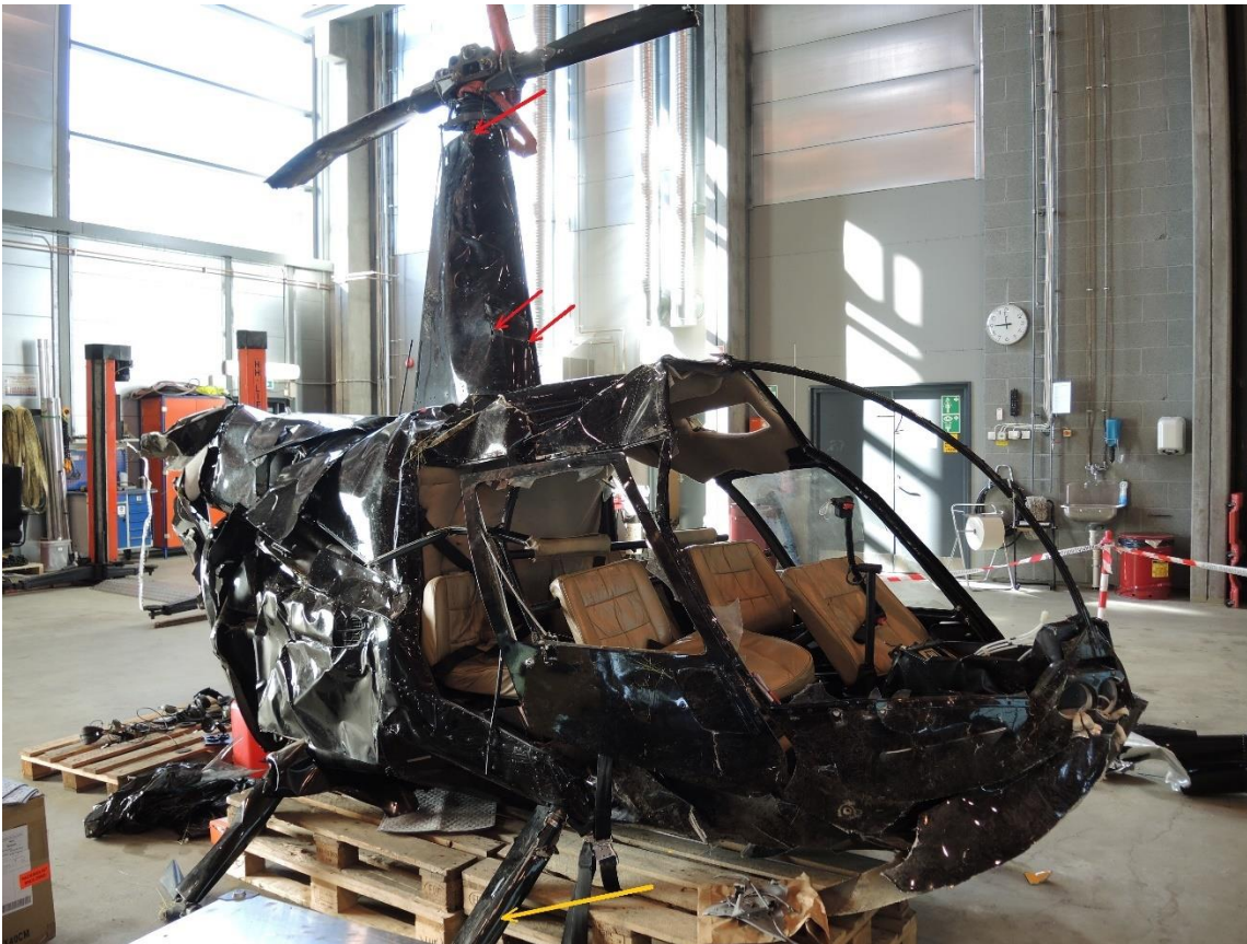
Figure 9: The damage to the right side of the helicopter photographed in the NSIA's hangar. The red arrows point to areas with melted aluminium. The yellow arrow points to scratch marks on the right forward landing gear leg. Photo: NSIA
