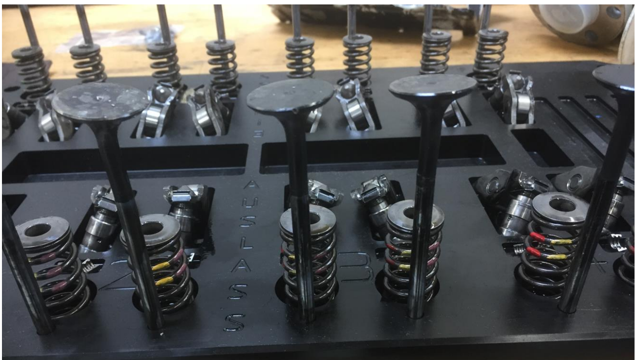
Figure 11: Exhaust valves from cylinders 2 and 3 with bent stems. Photo: NSIA
