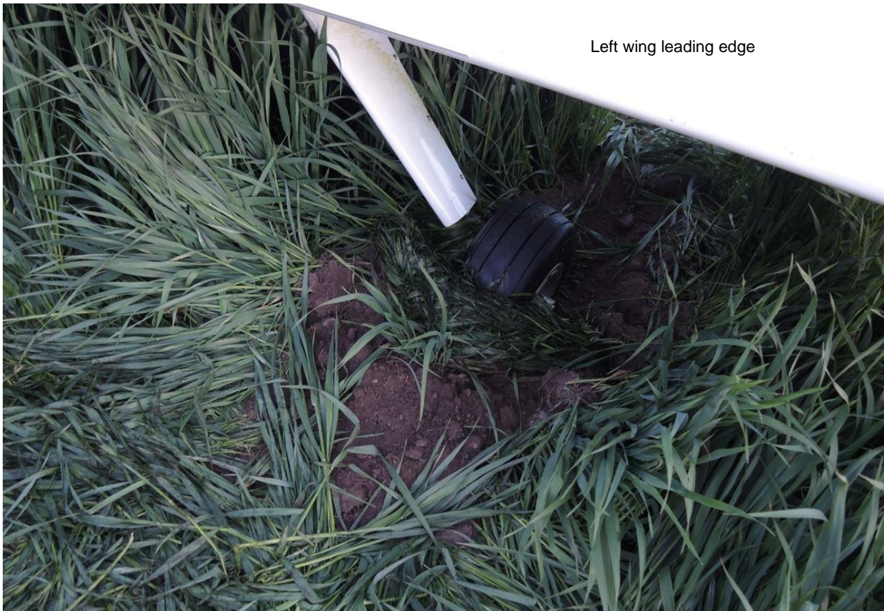
Figure 7: Deep tracks in the surface from the left main wheel. Photo: NSIA
