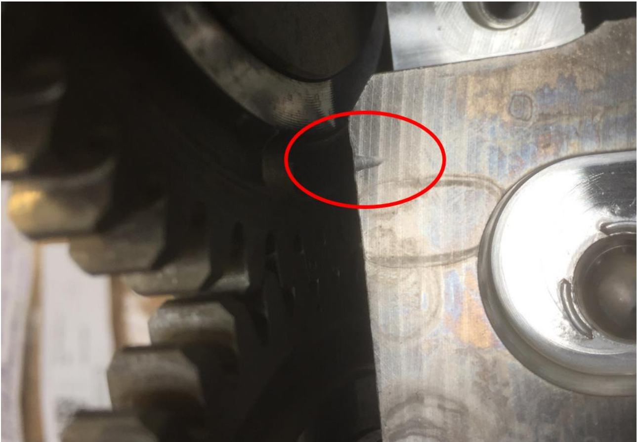
Figure 13: Marks left by the camshaft locking tool. Photo: NSIA
