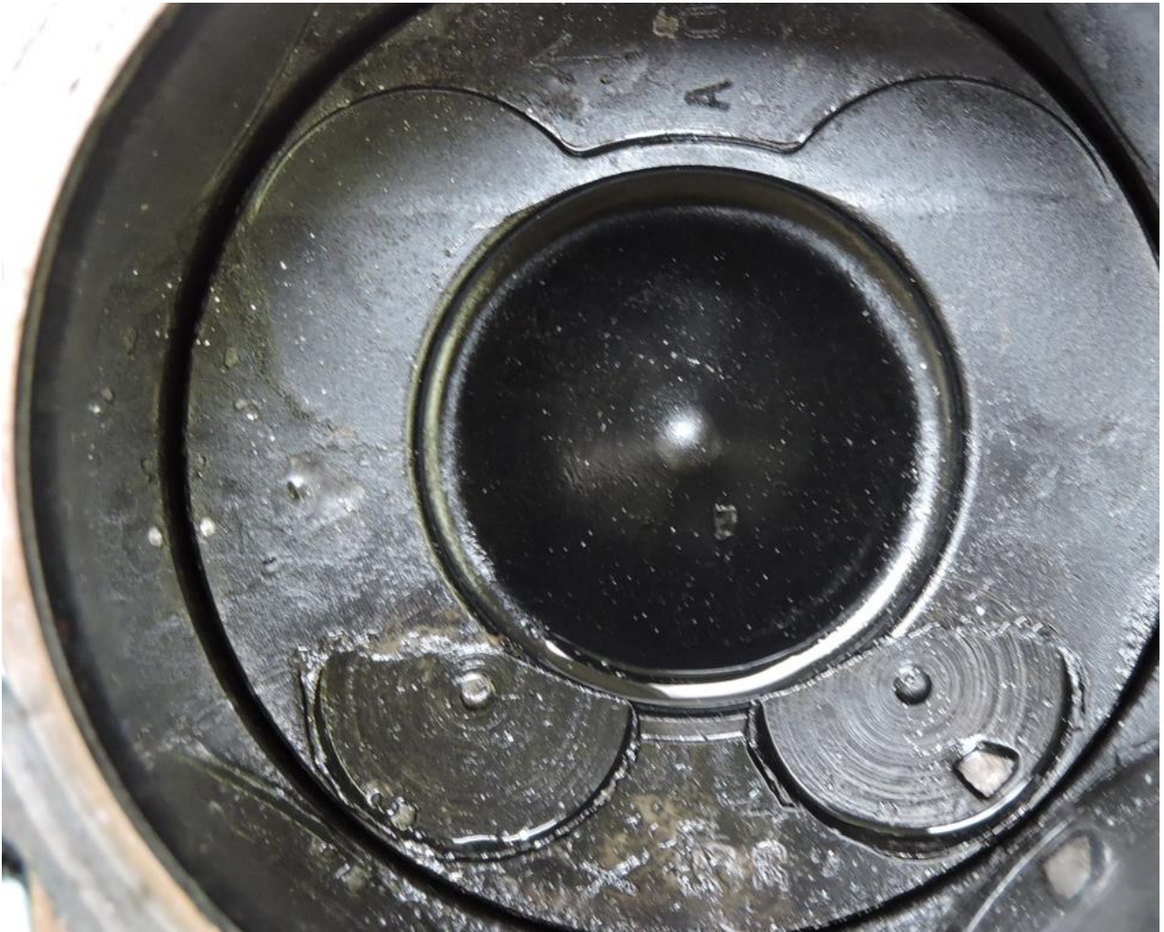
Figure 12: Imprints in piston crown 4 after impact with both exhaust valves (lower part of photo). Photo: Austrian Civil Aviation Safety Investigation Authority
