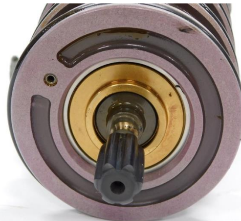
Figure 4: The oil pump and driveshaft with the Vespel spline adapter removed. The Vespel spline adapter slides on the driveshaft. Photo: Sikorsky/NSIA
