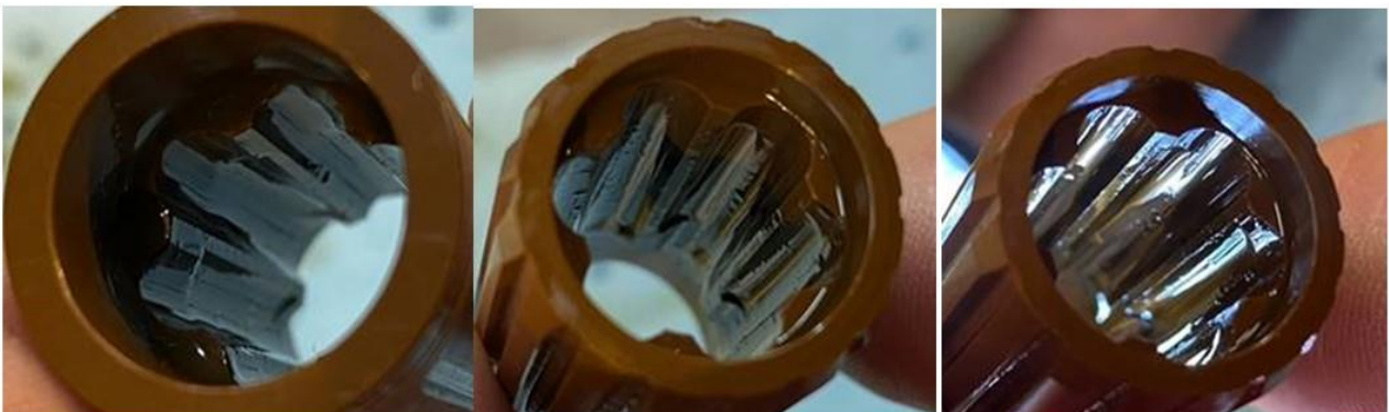
Figure 8: Photos of the removed Vespel spline adapters. The photo clearly demonstrates that spline adapter #1 is completely worn down internally. Wear can also be seen on spline adapter #2. Photo: Bristow/NSIA
