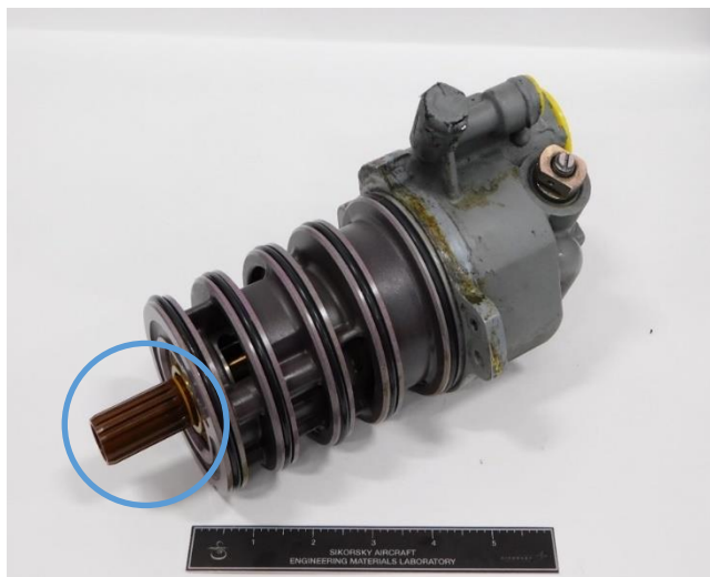
Figure 3: The oil pump. The Vespel spline adapter is marked with a ring. Photo: Sikorsky/NSIA
