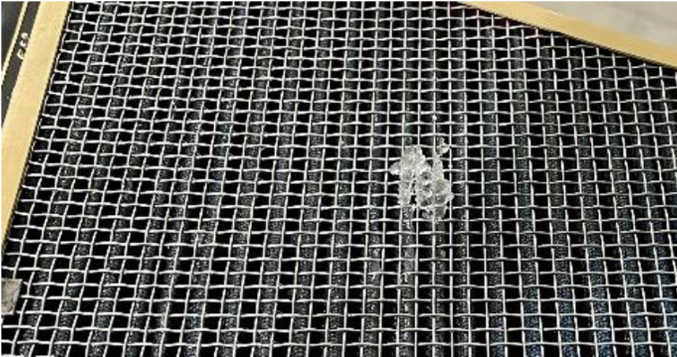
Figure 14: Ice build-up on the underside of the IBF filter. Photo: Airbus Helicopters / NSIA
