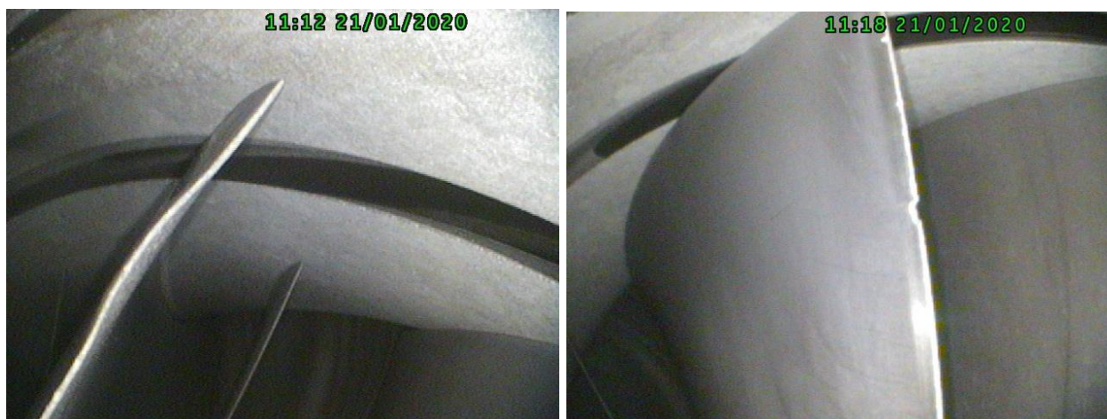
Figure 5: Borescope images showing damage to compressor blades caused by ice that came off the engine inlet and was sucked into the engine. Photo: Widerøe
