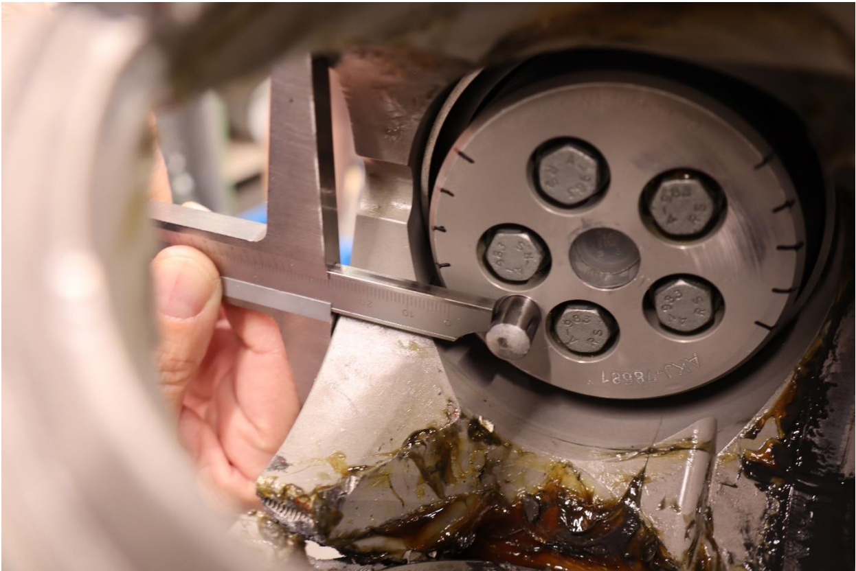
Figure 29: Measuring the distances between the blades' guide pins and the face of the propeller hub. Photo: BFU/NSIA
