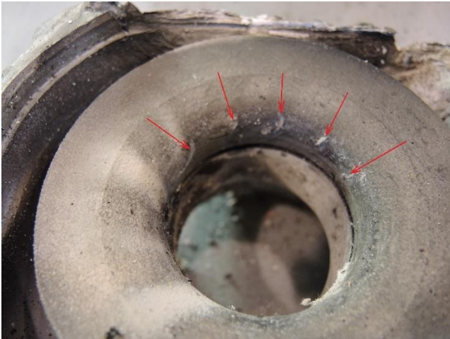
Figure 19: Compressor housing from the turbo for the right engine. The arrows point to damage to the housing from contact with the compressor rotor. Photo: NSIA
