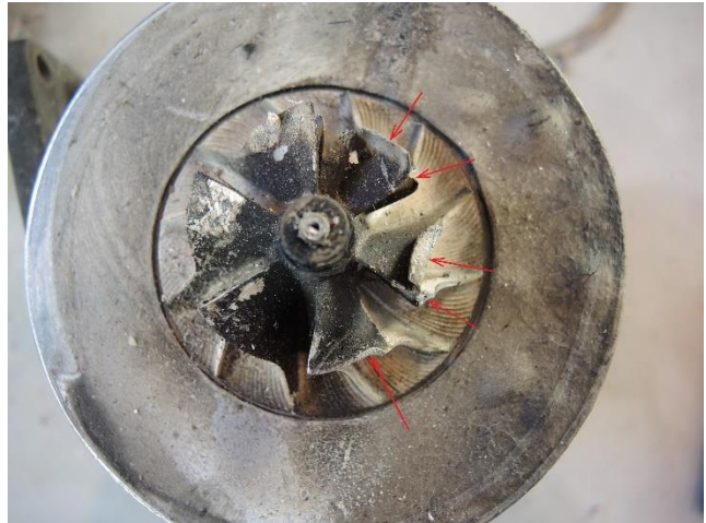
Figure 20: Compressor rotor from the turbo for the right engine. The arrows point to bent rotor blades. Photo: NSIA
