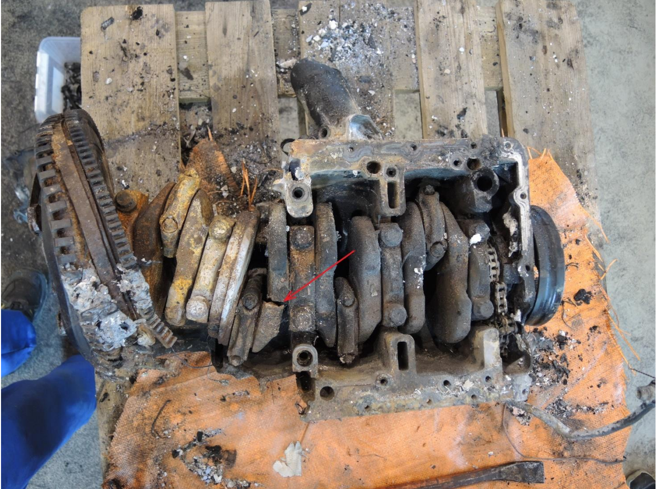
Figure 18: Damage to the left engine, viewed from below. The crankcase is largely crushed or missing. The red arrow points to where the crankshaft is broken. Photo: NSIA
