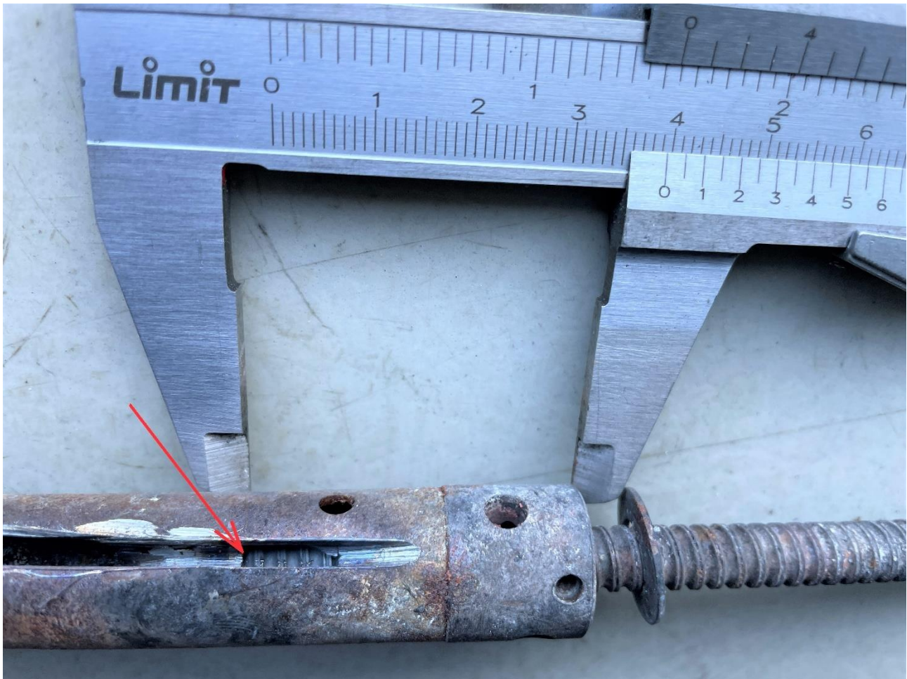
Figure 15: The rod for the flaps actuator on the left, with the jackscrew extending out to the right. The arrow points to the place where the screw has stopped against the end stop. Photo: NSIA
