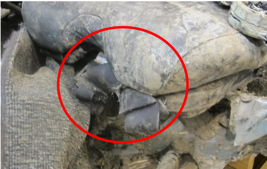
Figure 11: One of five straps for the front passenger seat was stowed underneath he seat. Photo: SHK
