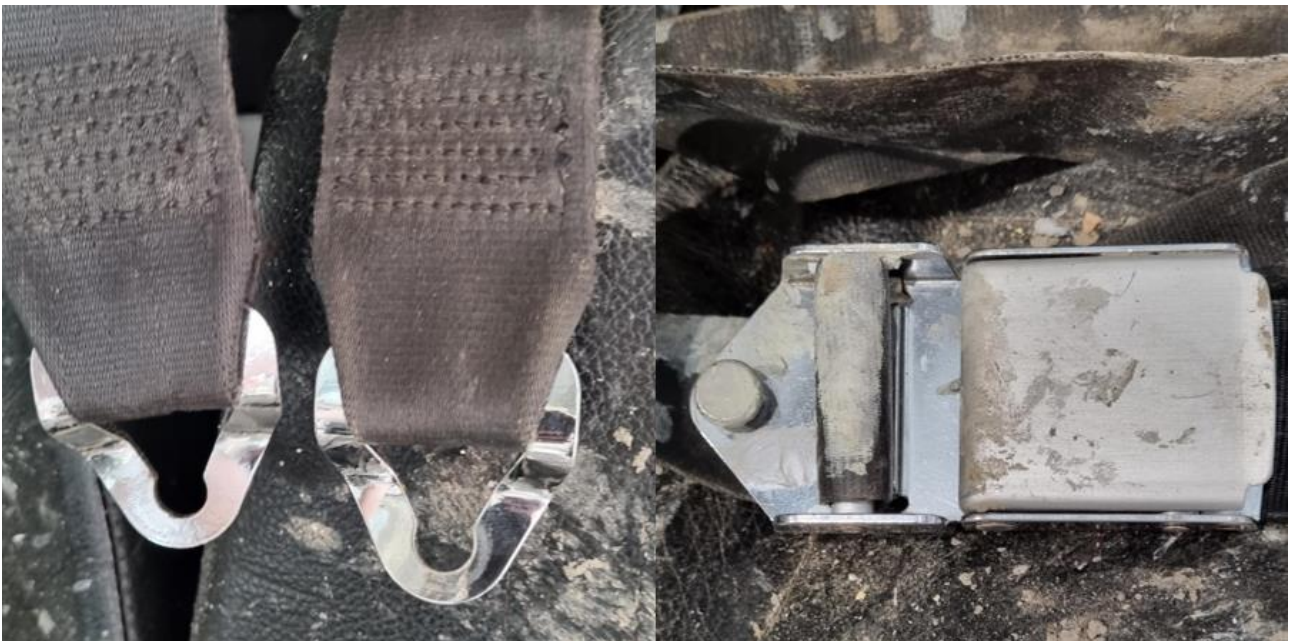
Figure 19: Foto of the safety harness of the passenger in the rear seat. There are no signs of paint on the shoulder strap, while a lot of paint can be seen on the lap strap. Both shoulder straps which are mounted in the same fixture was investigated to see if the passenger had used the wrong shoulder strap. Photo: NSIA
