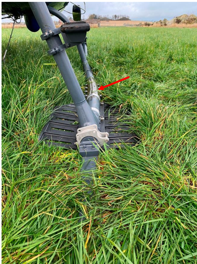
Figure 3: The right skid. The red arrow is pointing towards the bend: Photo: Helitrans/NSIA
