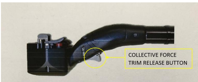
Figure 14: Collective with collective force trim release button. Photo: S-92 Pilot Training Manual / NSIA
