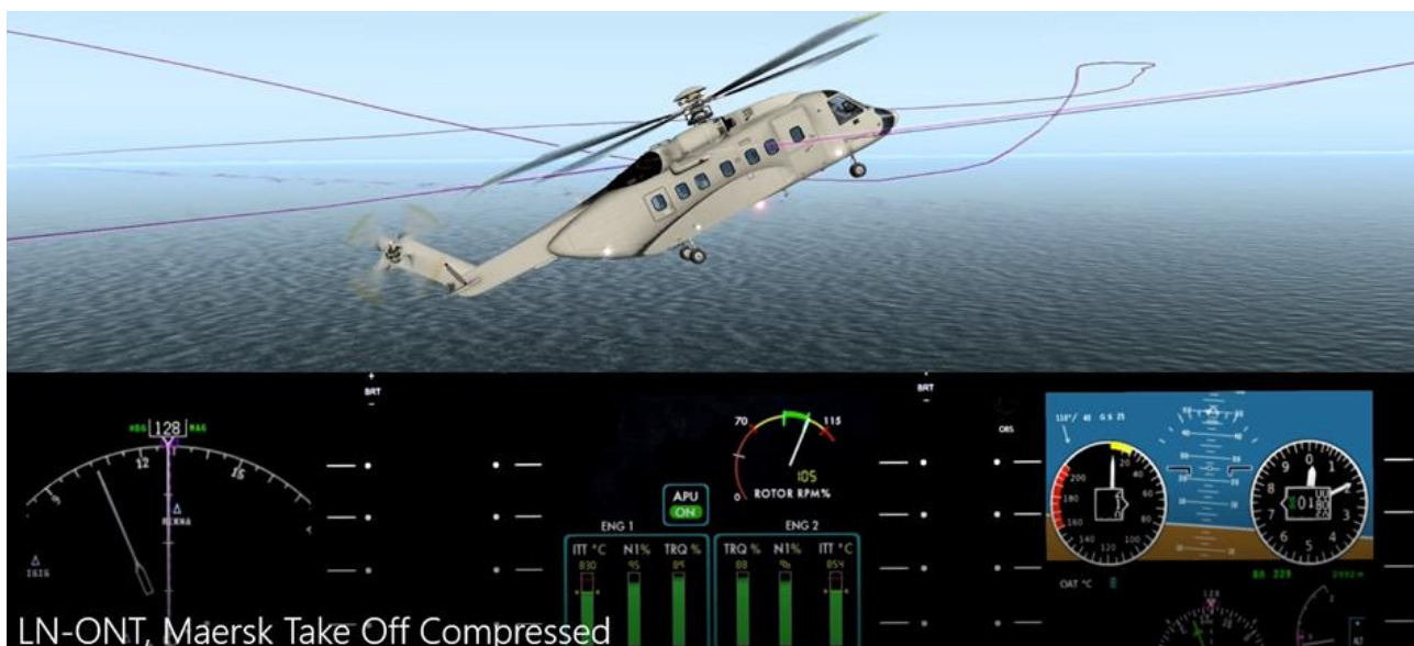
Figure 3: The highest pitch-up attitude after take-off exceeded 25° while the helicopter was accelerating rearwards and reached a ground speed of 49 kts. Animation: L3 Harris Technologies UK / NSIA. Source: LN-ONT CVFDR
