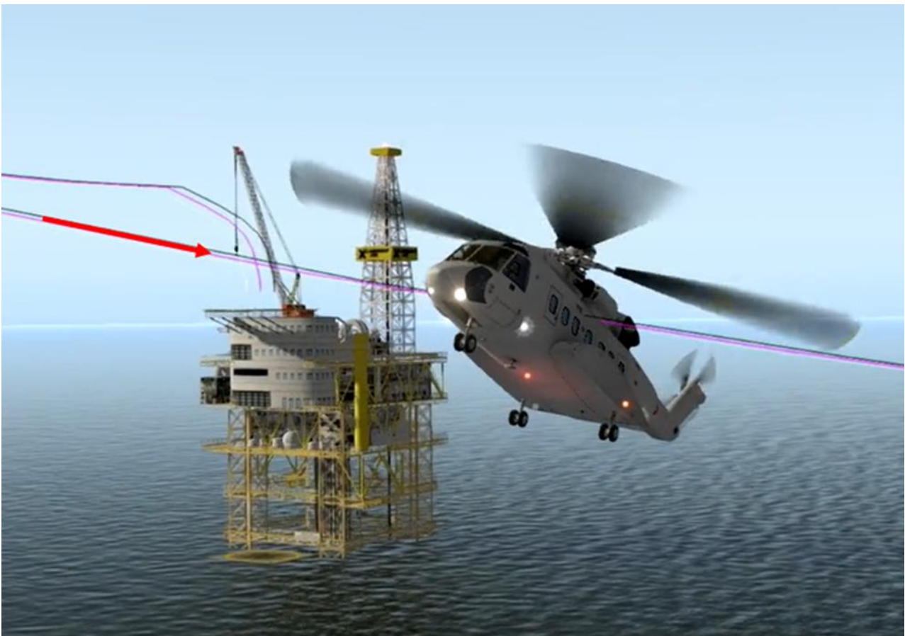
Figure 6: Animation of LN-ONT passing the oil installation while the helicopter flies backwards. (The oil installation is an illustration and not identical to Maersk Invincible). Animation: L3 Harris Technologies UK / NSIA. Source: LN-ONT CVFDR
