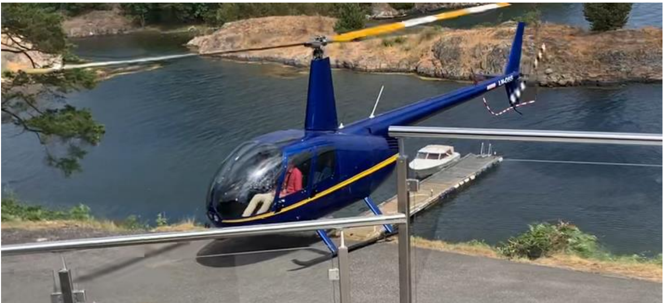
Figure 6: Stills from the video footage showing that when the helicopter landed, a large section of the skids was outside the edge of the tarmacked area. Photo: Private video / NSIA
