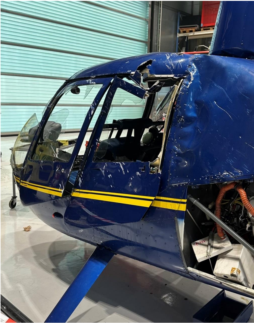
Figure 5: The illustration shows the left side of the cabin that was under water. The battery is the white box in the lower right-hand corner of the photo. Photo: NSIA
