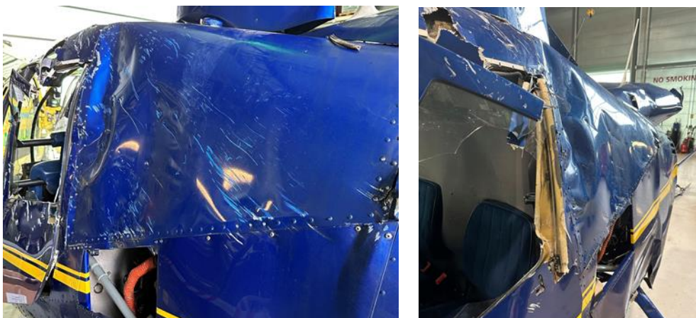
Figure 8: Damage to the left fuel tank. Photo: NSIA
