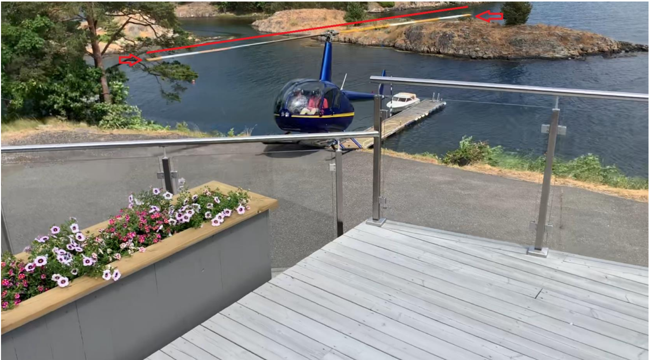
Figure 7: Stills from the video footage showing the helicopter about to tip down onto the slope. The red arrows indicate that the helicopter had an almost flat pitch (minimal lift from the rotor blades). The line shows virtually no coning of the main rotor. Photo: Private video, annotation by NSIA
