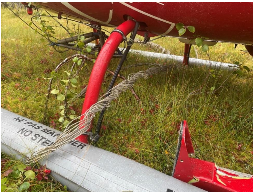
Figure 7: The aluminium wires wrapped around the helicopter's right skid with floats after the emergency landing on the marsh. Photo: Heli-Team/NSIA
