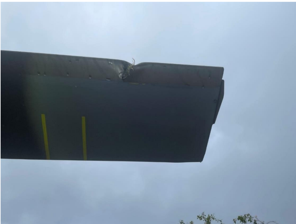
Figure 6: The rotor blade that cut the power cable. Photo: Heli-Team/NSIA
