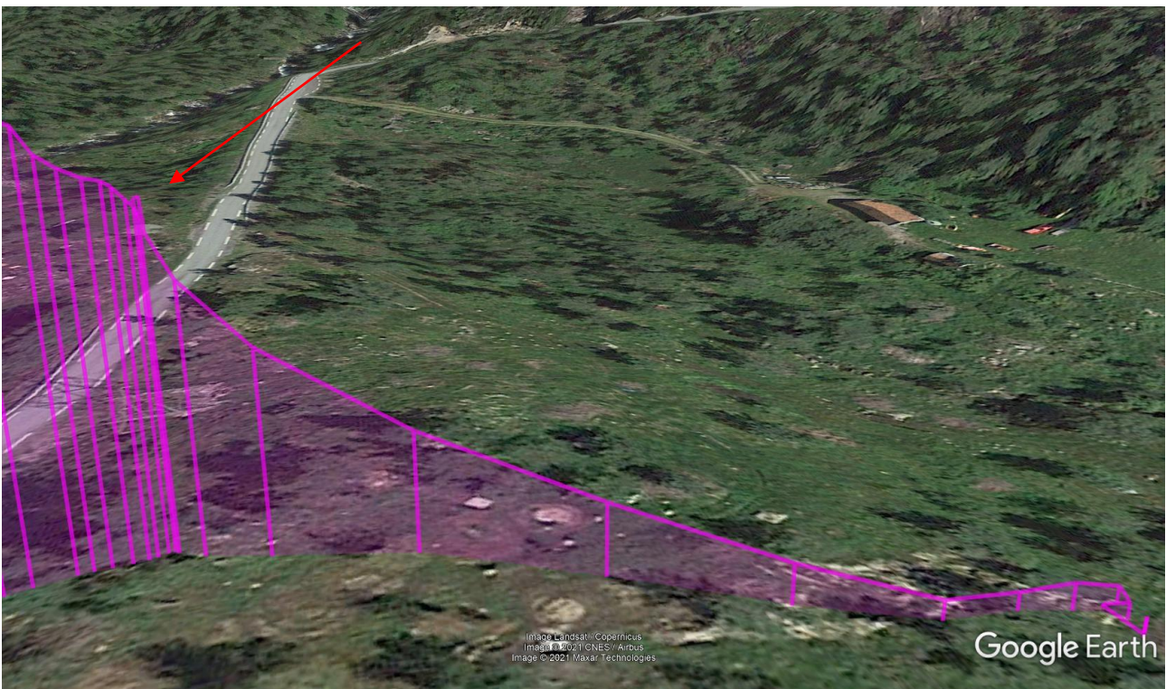
Figure 16: The illustration shows the last movements and crash site of the helicopter. The red arrow indicates a vertical movement just above pylon foundation 49. Each vertical reference line represents one second. The last four seconds of recording is judged as not reliable. Source: Air Navigation Pro / Google Earth / NSIA
