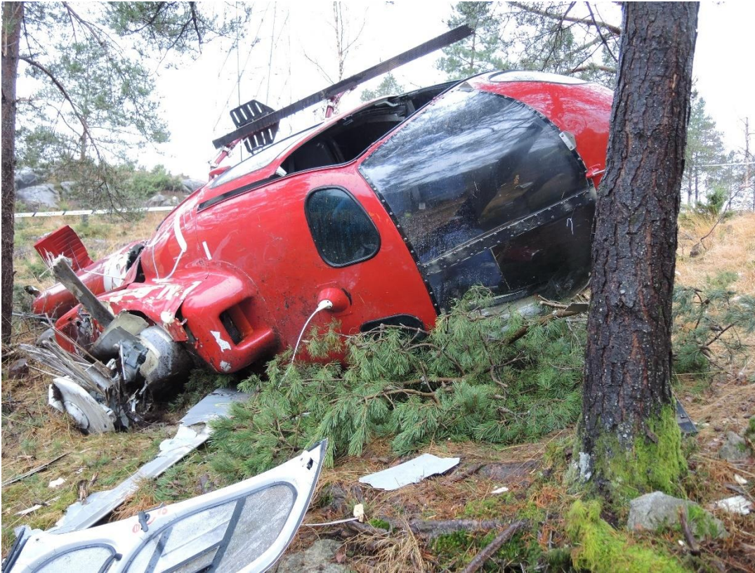
Figure 12: The helicopter wreck looking southwest. One of the rotor blades has been coiled around the rotor mast. Photo: NSIA
