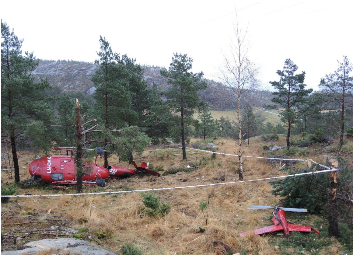
Figure 3: The helicopter's final position about 50 metres east of pylon foundation 49. The tail rotor with the vertical stabiliser on the right. Photo looking east, with pylon foundation 49 behind the photographer. Photo: NSIA
