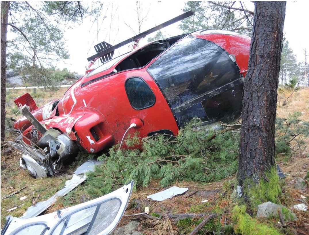
Figure 12: The helicopter wreck looking southwest. One of the rotor blades has been coiled around the rotor mast. Photo: NSIA
