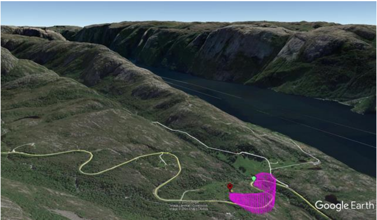
Figure 15: The illustration is seen in a 135° direction. The last flight is illustrated on the basis of data downloaded from Air Navigation Pro. The starting point is indicated by a green pin and the crash site by a red pin. Source: Air Navigation Pro / Google Earth / NSIA
